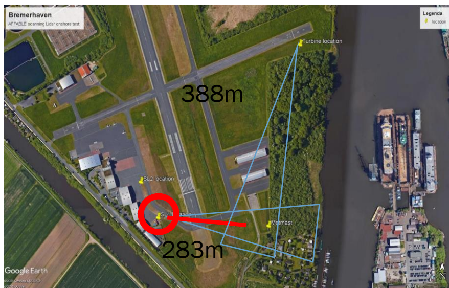
Onshore campaign at Bremerhaven: LiDARs positioning with relation to met mast. Source: AFFABLE
