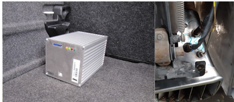
Figure 2: Example of the system installed on the vehicle. On the left, the SEMS central unit where the data is gathered and stored. On the right: the welding of the sensors on the exhaust.
