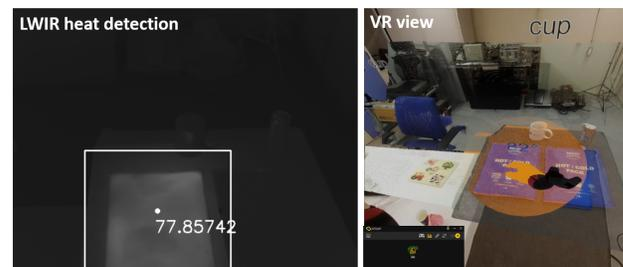
**Figure 7: Left: Detection of high-temperature object from LWIR frame. Right: 3D VR rendering of the high-temperature object as a pointcloud from stereo feed, and as a heat-sphere, through LWIR-stereo camera calibration with accurate temperature label display (77°C). Operator’s hand is colliding with the sphere in VR to grasp the high-temperature object and the corresponding temperature is rendered through bHaptics interface on ThermoReal glove.**
