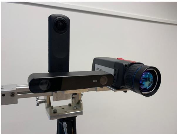
Figure 2: Fixed frame sensor suite including long-wave infrared sensor with 45° lens from FLIR, 360° Theta Ricoh Z1 camera from Ricoh, and stereo camera Zed2i from StereoLabs
