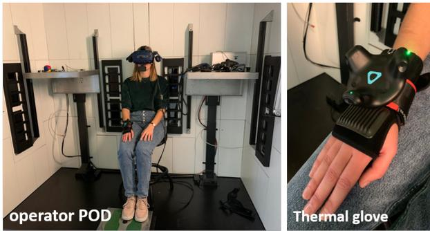
**Figure 4: Left: Operator sitting inside the Sensiks POD, surrounded by six built-in heaters of which four are visible (black panels), and wearing a virtual-reality head-mounted display and a thermal glove. Right: The operator's hand wearing the ThermoReal glove with a Vive tracker for hand tracking.**
