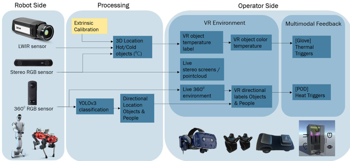
Figure 1: System architecture diagram. The robot side is represented by its sensor suite and the operator side by the different rendering modalities.
