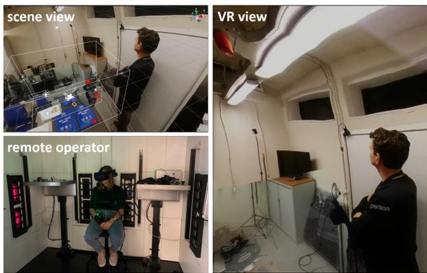
**Figure 6: Testing ambient temperature perception with a recipient standing at the left of the robot’s sensor suite and the corresponding leftmost POD heater activated. Classification label ('person') is visually rendered in VR**
