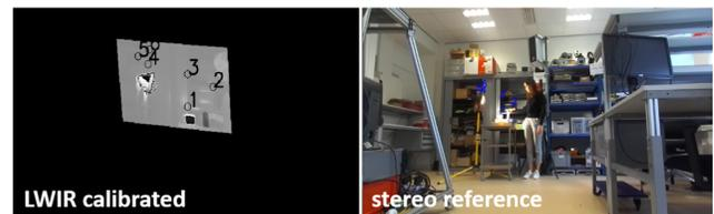
Figure 3: Left: LWIR image warped according to estimated homography matrix, through six correspondences between LWIR and stereo images. Right: Reference left stereo image with the six established correspondences.
