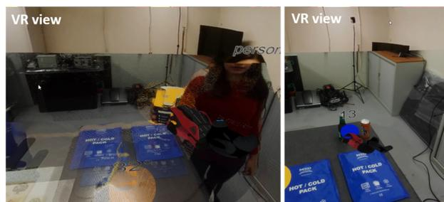
**Figure 8: Left: VR operator grasping hot beverage cup with human recipient (visual rendering as pointcloud) and perceiving its temperature. Right: VR grasping a cold beverage from the testing table (visual rendering as stereo screens) perceiving its temperature.**
