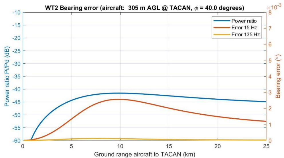
Figure 7.17 Bearing error in the 15 Hz and 135 Hz signal. Flight trajectory altitude is 305 m AGL and angle \phi = 40^\circ .
