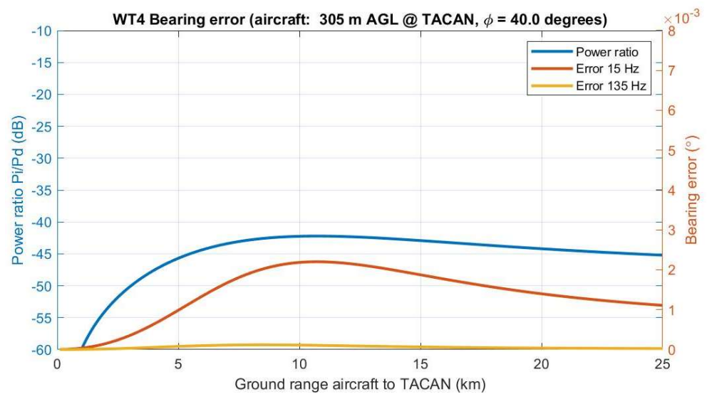
Figure 7.27 Bearing error in the 15 Hz and 135 Hz signal. Flight trajectory altitude is 305 m AMSL and angle \phi = 40^\circ .
