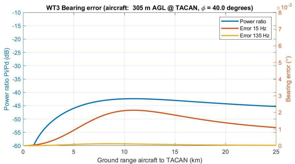
Figure 7.22 Bearing error in the 15 Hz and 135 Hz signal. Flight trajectory altitude is 305 m AGL and angle \phi = 40^\circ .
