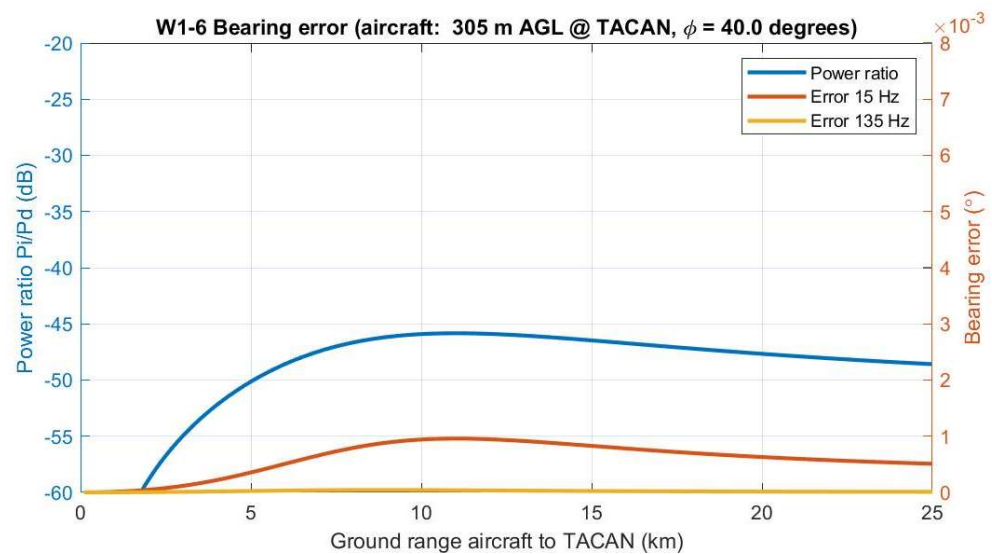
Figure 7.7 Bearing error in the 15 Hz and 135 Hz signal. Flight trajectory altitude is 305 m AGL and angle \phi = 40^\circ .
