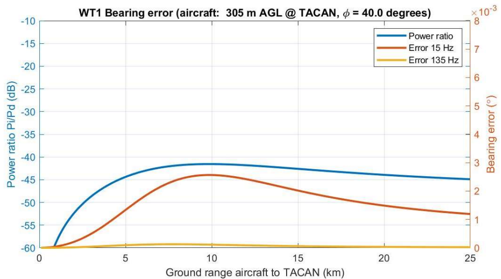
Figure 7.12 Bearing error in the 15 Hz and 135 Hz signal. Flight trajectory altitude is 305 m AGL and angle \phi = 40^\circ .
