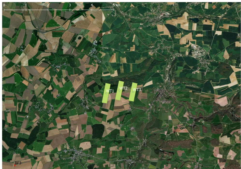
Figure 4.7 The combined raised threshold regions for all nine newly planned turbines in the range of the STAR 2000 PSR at Florennes with the WFF CFAR processing enhancement.
