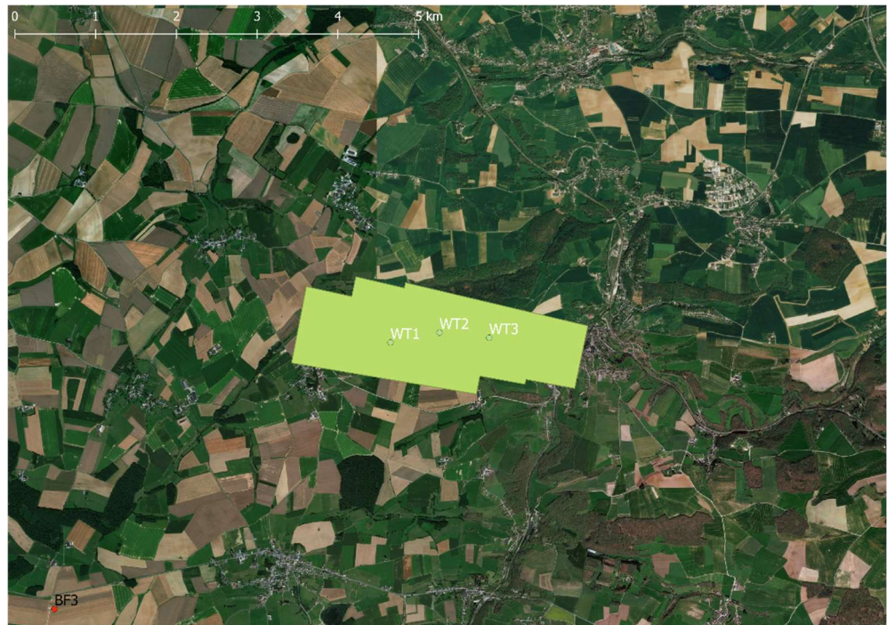
Figure 4.6 The combined raised threshold regions for all nine newly planned turbines in the range of the STAR 2000 PSR at Florennes without the WFF CFAR processing enhancement.
