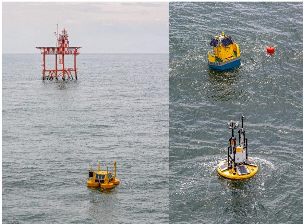
Figure 5 Aerial captures of three floating LiDAR systems during a validation campaign at LEG platform photo taken by Flying Focus.
