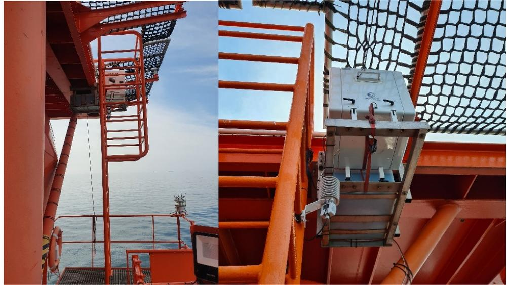
Figure 7 Views of newly installed LiDAR unit for the scheduled replacement period in 2021 onwards.
