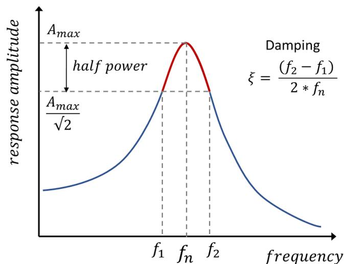
Figure B-1 Graphic representation of the half-power bandwidth method for structural damping estimation.
