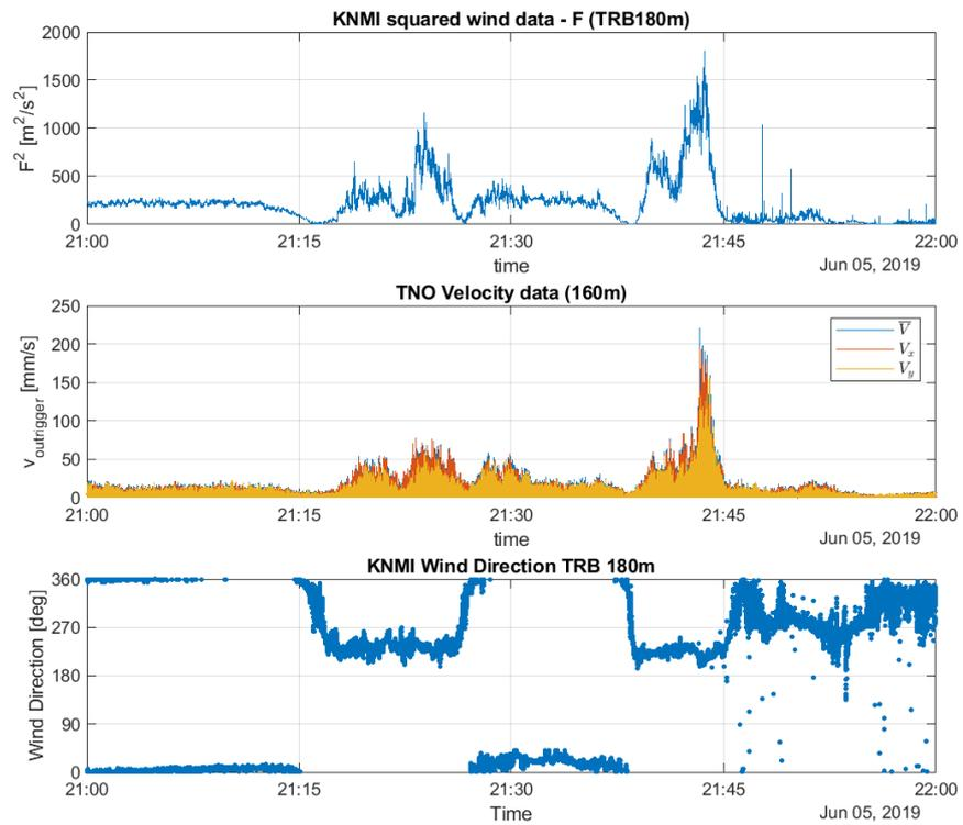
Figure 3-5 Squared wind velocity (top) and direction (bottom) measured from the KNMI sensors at 180m and the velocity of the sensors on the outriggers at 160m (middle) during the gust event of the 5<sup>th</sup> of June 2019 (21:00 – 22:00, UTC time).
