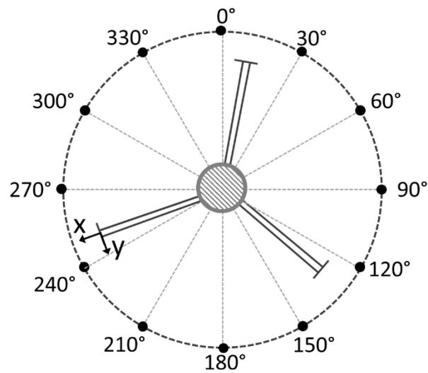
Figure 2-2: Orientation of outrigger with respect to wind direction and orientation of the local X and Y axes of the sensors.
