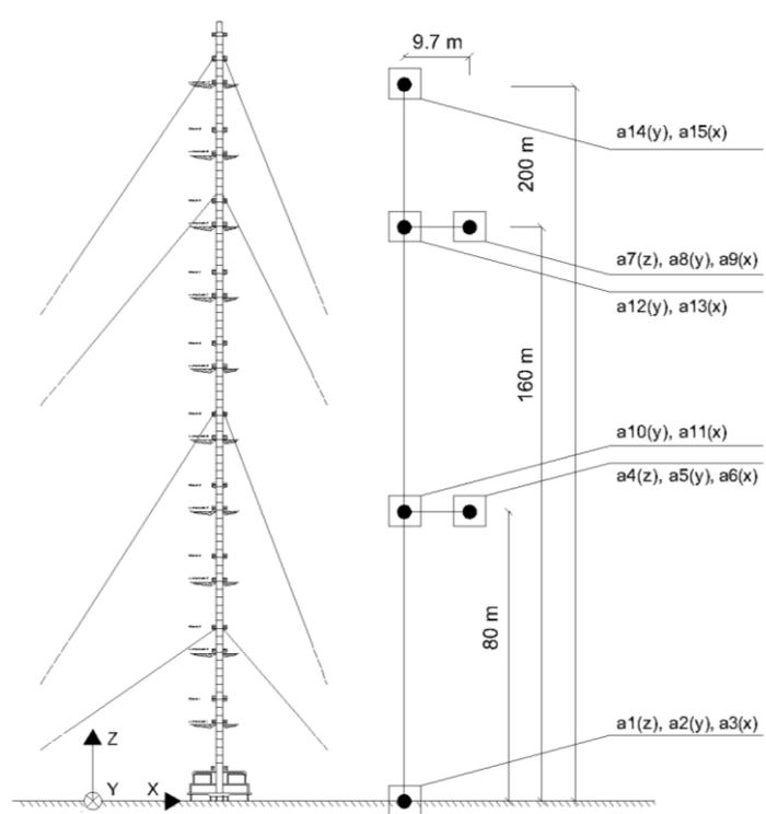
Figure 2-1: overview of acceleration sensor locations on the meteorological tower.
