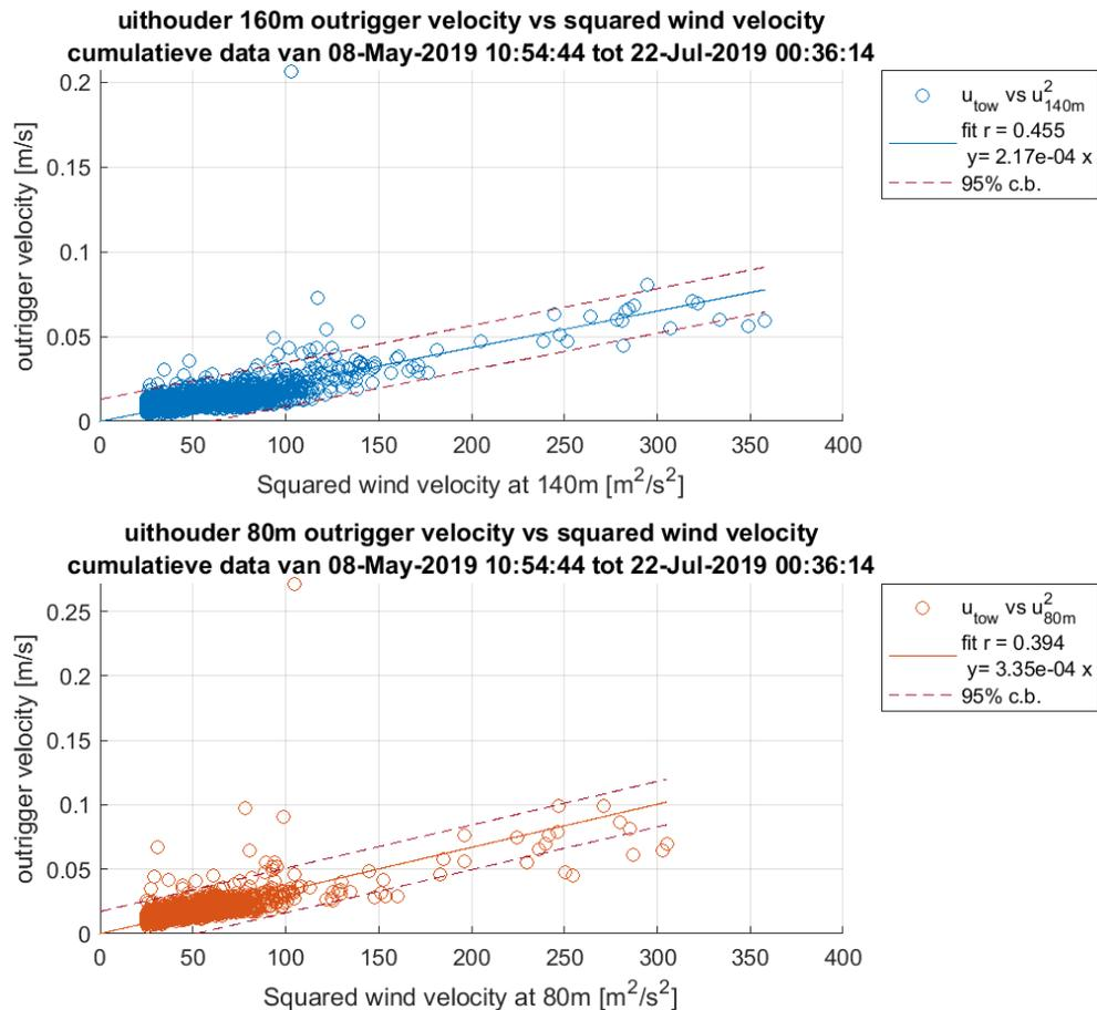
Figure 3-3 Maximum hourly outrigger velocity versus the squared mean wind speed for the period between the 8<sup>th</sup> of May 2019 and the 22<sup>nd</sup> of July 2019 for the outrigger at 160m (top) and the outrigger at 80m (bottom). The plot includes a linear fit (blue line) and a 95% confidence interval (dotted red lines).
