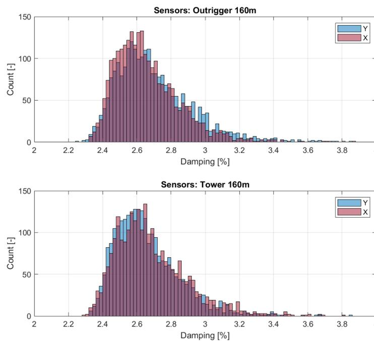
Figure B-2 Damping percentage estimated with the half-power bandwidth method for each of the measurement of Period 1 for the sensors on the outrigger (top) and the tower (bottom) at 160m in X and Y direction.
