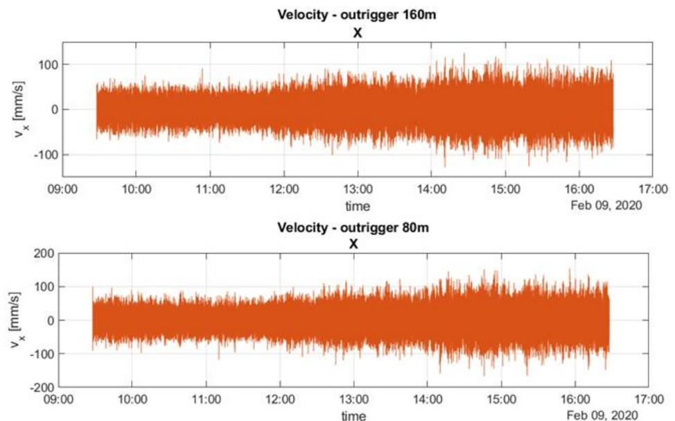
Figure 4-2 Outrigger X velocities at 160m (top) and 80m (bottom) between the 9:00 and 17:00 (UTC time) on the 9<sup>th</sup> of February 2020.
