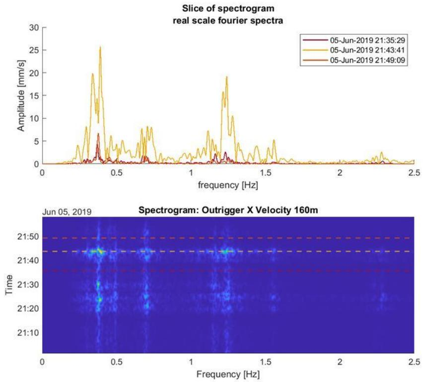
Figure 3-6 (bottom) Spectrogram of the outrigger velocity in X direction and (top) 3 cross section of the spectrogram: before, during and after the gust event. The spectrogram was obtained using time windows of 164 seconds to achieve a higher frequency resolution.
