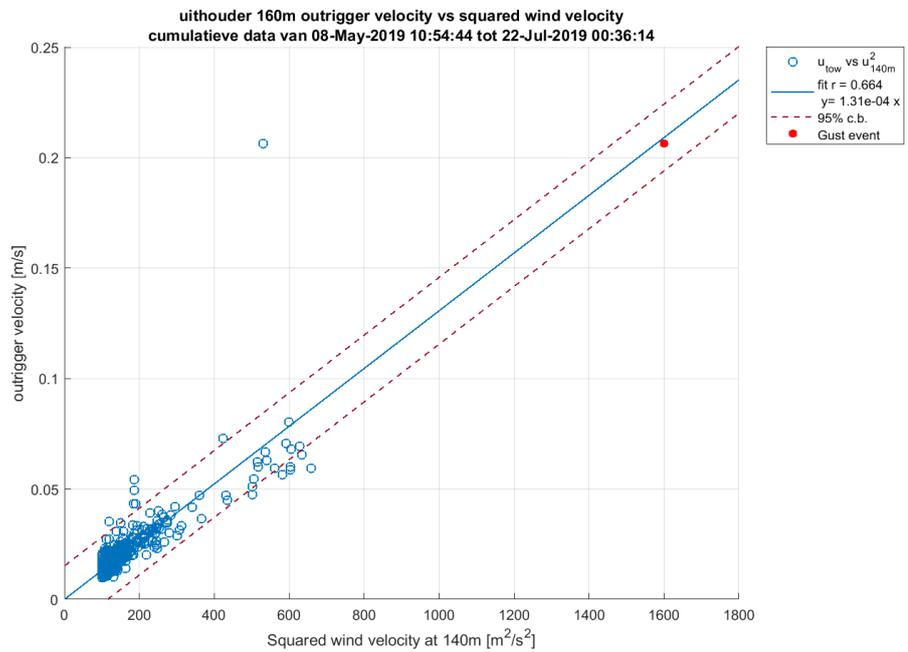
Figure 3-7 Maximum hourly outrigger velocity against the squared peak wind velocity for the period between the 8<sup>th</sup> of May 2019 and the 22<sup>nd</sup> of July 2019 for the outrigger at 160m (top) and the outrigger at 80m (bottom). The plot includes a linear fit (blue line) and a 95% confidence interval (dotted red lines). The blue dots use the peak wind velocities from
