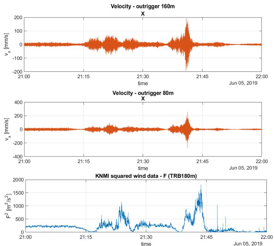
Figure A-1 Outrigger X-velocity at 160m (top) and 80m (middle) and squared wind velocity measured from the KNMI sensors at 180m (bottom) during the gust event of the 5<sup>th</sup> of June 2019 (21:00 – 22:00, UTC time).
