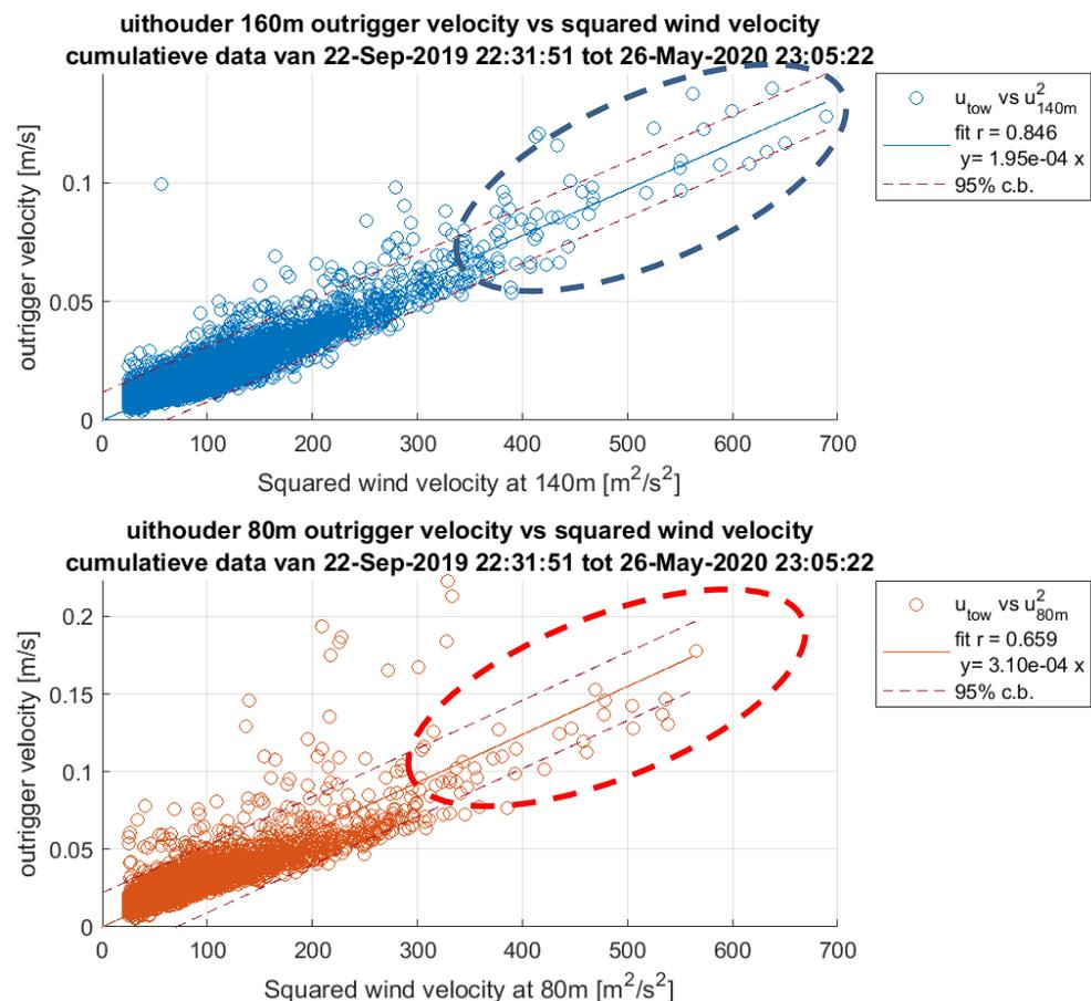
Figure 4-3 Maximum hourly outrigger velocity against the squared mean wind speed for the period between the 22<sup>th</sup> of September 2019 and the 26<sup>th</sup> of May 2020 after removing the outliers for the outrigger at 160m (top) and the outrigger at 80m (bottom). The plot includes a linear fit and a 95% confidence interval (dotted red lines).
