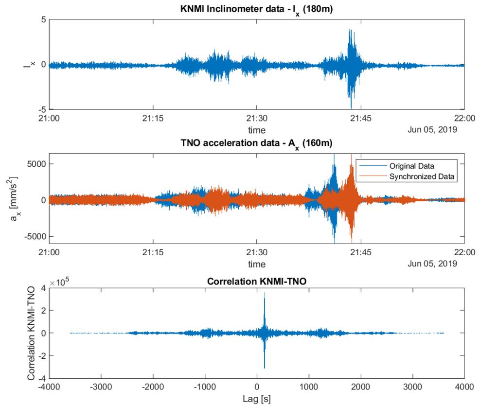
Figure A-2 Inclinator data measured from the KNMI sensors at 180m (top), X-acceleration of the outriggers at 160m (middle) original (blue) and synchronised (orange) and the correlation between the inclinometer data and original acceleration data (bottom) during the gust event of the 5<sup>th</sup> of June 2019 (21:00 – 22:00, UTC time).
