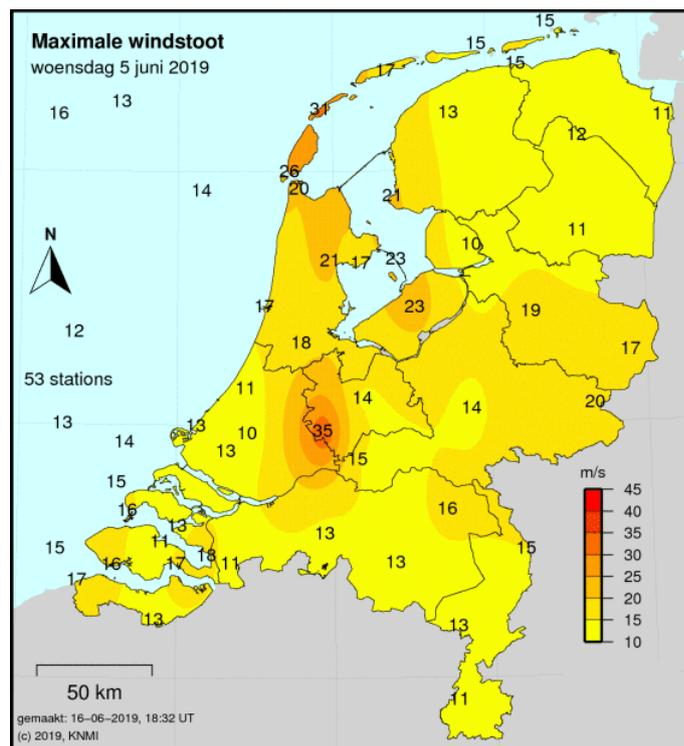
Figure 3-1 Contour of the maximum wind gust observed on the 5<sup>th</sup> of June 2019. The largest wind gust of 35m/s is recorded at the site of the Cabauw tower.
