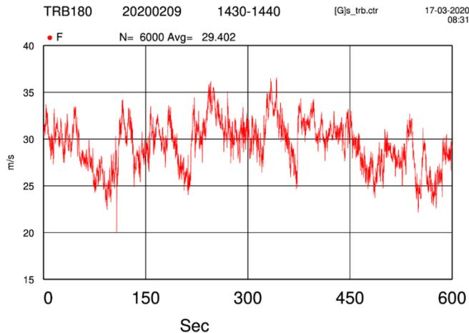
Figure 4-1 Horizontal component of the wind velocity measured by the KNMI sensors at the Cabauw tower at 180m height on the 9<sup>th</sup> of February 2020, between 14:30 and 14:40 (UTC time).
