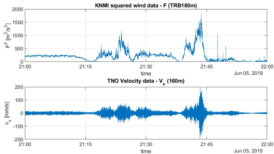
Figure 3-4 Timeseries measured in the gust event of the 5<sup>th</sup> of June 2019 (21:00 – 22:00, UTC time): (top) the squared wind velocity at 180m, and (bottom) the velocity in X-direction of the outriggers at 160m.
