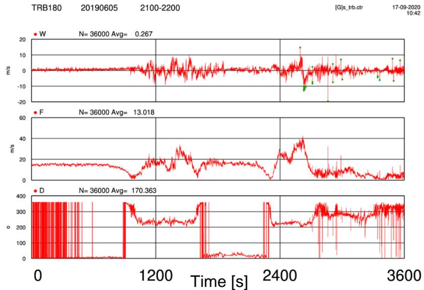
Figure 3-2 Time series measured by the KNMI on the Cabauw tower at 180m height on the 5<sup>th</sup> of June 2019, between 21:00 and 22:00 (UTC time): (top) vertical wind velocity, (middle) horizontal wind velocity, (bottom) wind direction of the horizontal wind velocity
