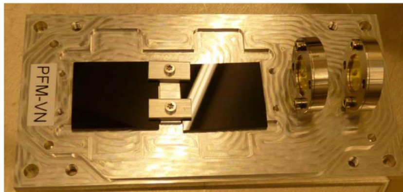
Figure 6-1 Sample holder used for PAC and MOC monitoring
