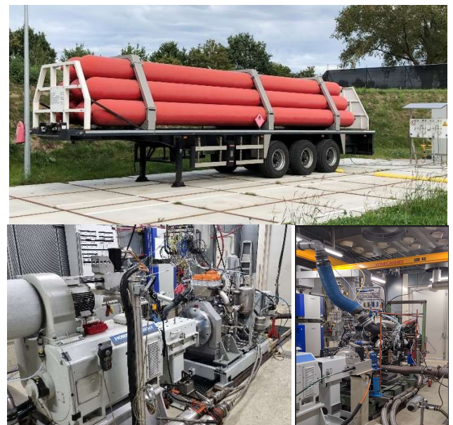
Fig. 1 Hydrogen infrastructure and test facilities at TNO in Helmond, The Netherlands. Compressed hydrogen is stored in tube trailer(s) feeding up to four individual test cells capable of running multi-cylinder engines up to 700 kW and heavy-duty single-cylinder engines.
