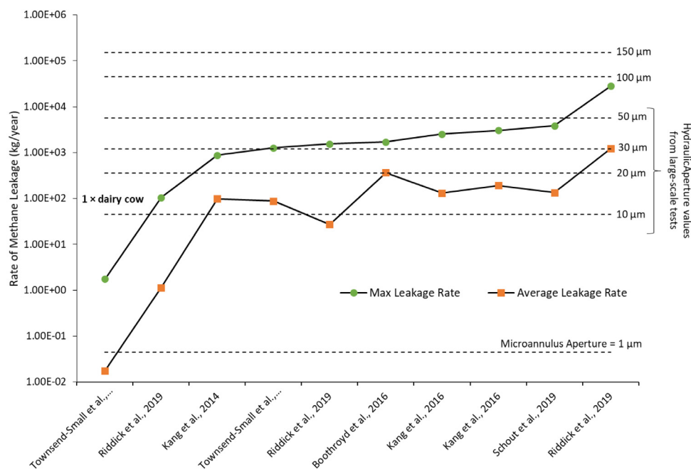
Fig. 11. Average and max leak rate measurements from various datasets compared to the calculated leakage rates using Eq. (7) (shown as dashed lines).
