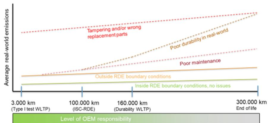
Figure 3-1: A schematic representation of the increase in emissions from gasoline cars due to various causes (TNO Report 2019 R10534). The manufacturer has less and less responsibility for these increases as mileage increases.
