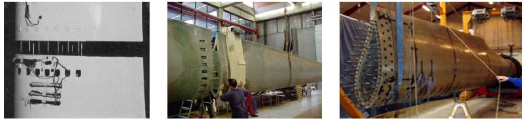
Figure 2-2: Prototypes of segmented blades using T-bolt joints [4]
