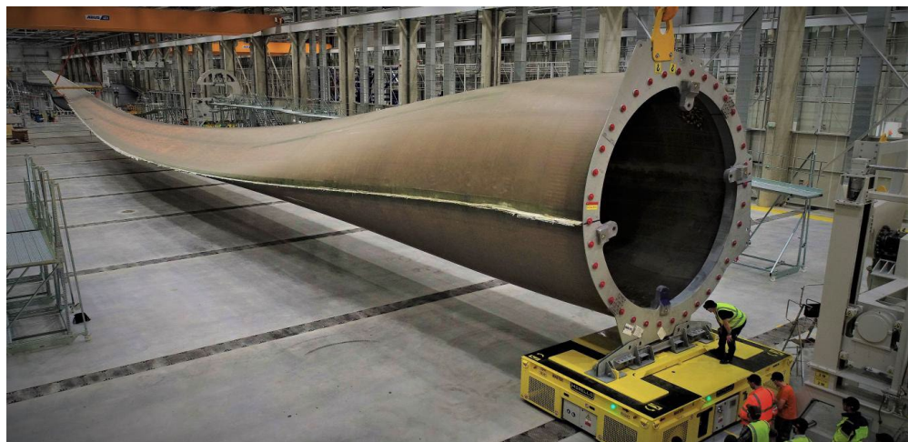
Figure 3-7 Blade handling exerts non-conventional loads on blades (source: https://www.ge.com/news/reports/extreme-measures-107-meters-worlds-largest-wind-turbine-blade-longer-football-field-heres-looks-like )
