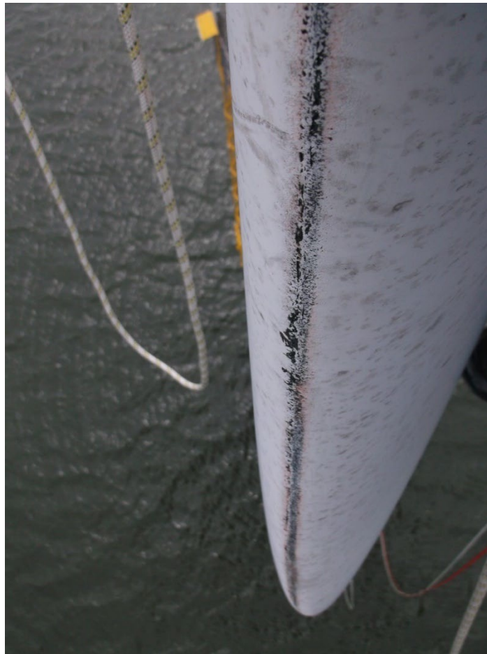
Figure 2-1: Blade surface and leading edge degradation due to pitting and erosion [2]
