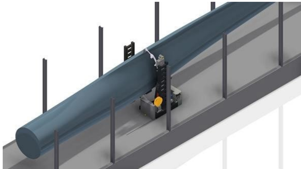
Figure 3-6 Automated blade coating (source: https://www.qlayers.com/bl8robot.html )
