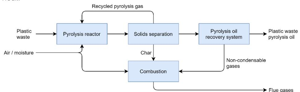
Figure 21 Plastic waste pyrolysis process in details
