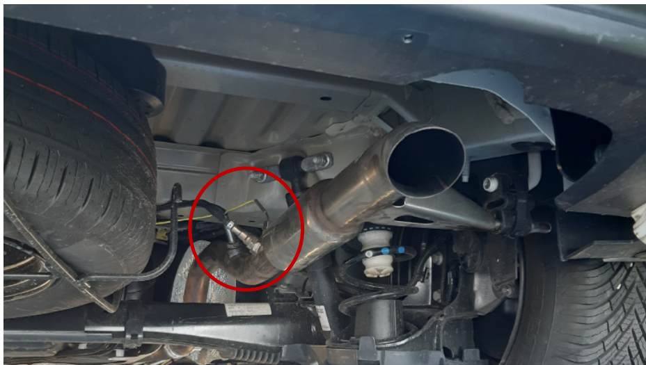
Figure 2.1: A NH 3 , a thermocouple and a NO x sensor installed at the end of an exhaust pipe.
