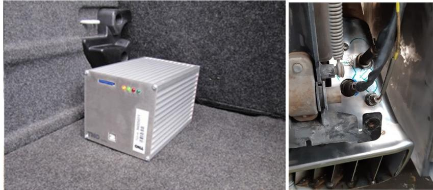
Figure 2: Smart Emissions Measurement System (SEMS), with sensors in the exhaust
