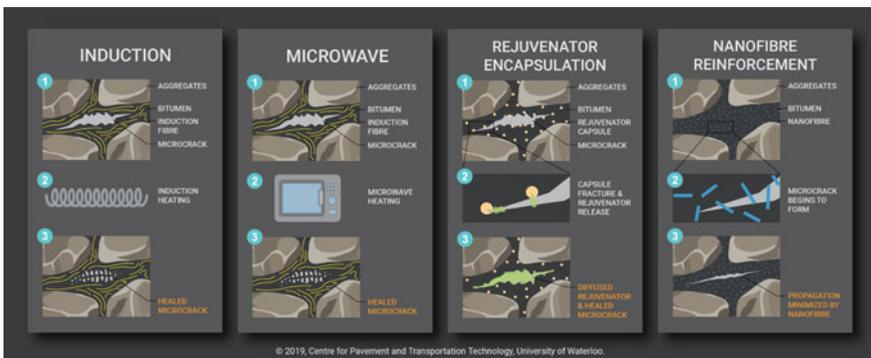
**Fig. 1** Different approaches to introduce additional self-healing performance (extrinsic) to bituminous materials
