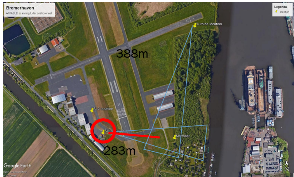
Figure 3: LiDARs setup with respect to the met mast. Scanning patterns are qualitatively represented in blue lines.
