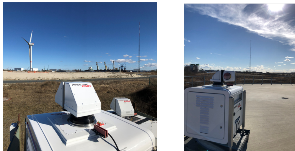
Figure 2: LiDARs at the Bremerhaven test field site. Image copyrights Fraunhofer. On the left, the western scanning and staring LiDARs. On the right, the northern scanning LiDAR.
