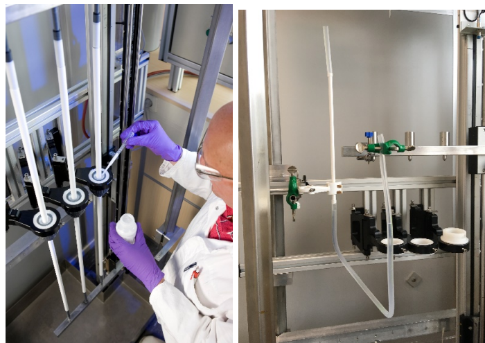
Figure 6: Set-up for coating on the outside (left) and inside (right) of tubular supports.
