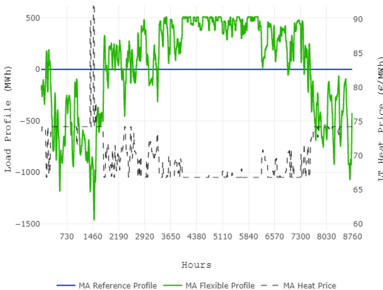
Fig. 18. Daily moving average of hot-water buffer load profile and the respective heat prices in the LT heat network.
