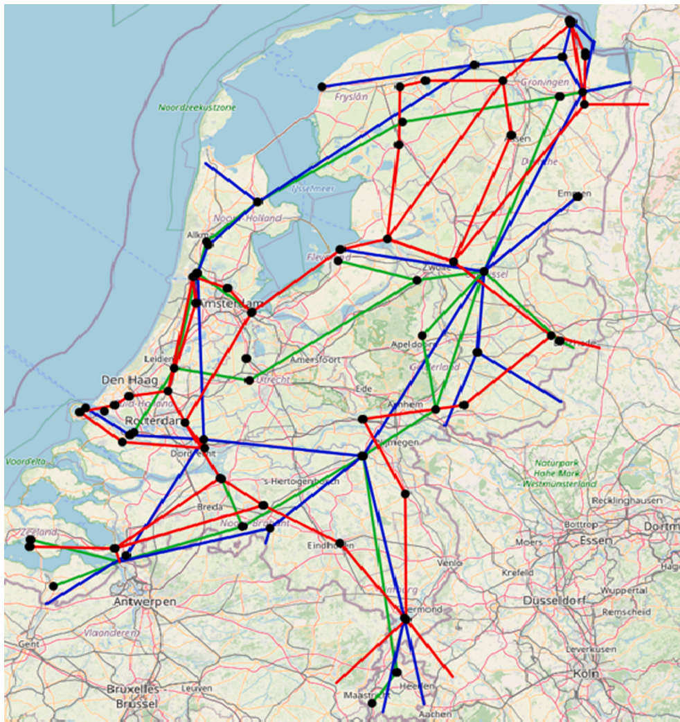
Fig. 3. Dutch transmission network topologies of electricity (red), hydrogen (blue) and methane (green) systems in 2050 [13,79].
