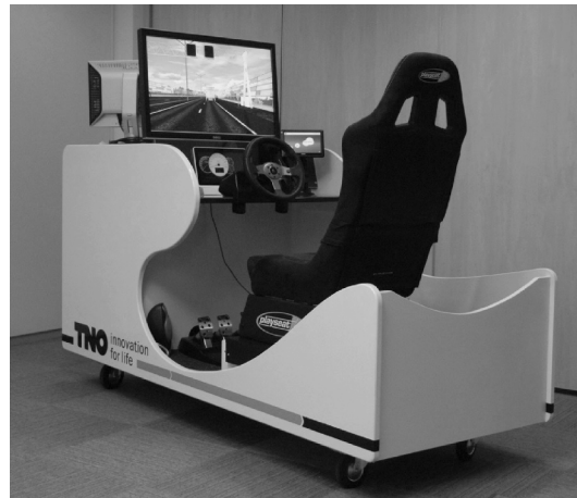
Fig. 2. Image of the route-choice driving simulator of TNO used in this experiment.
