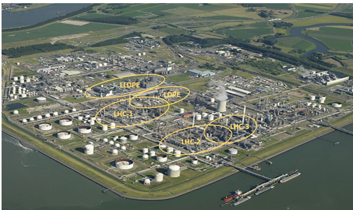
Figure 2 Aerial view of Dow chemical plants in the Terneuzen site with the locations of the LLDPE and LDPE production and the crackers where the Low Hydro Carbons (LHC) are produced (Dow, 2020b).
