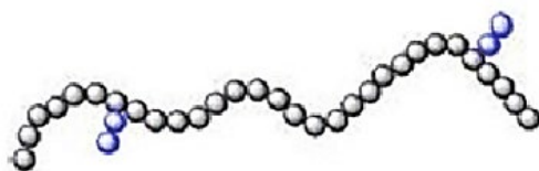
Figure 10 HDPE structure with the main carbon chain in black and the side branches in blue (Graziano et al., 2019)
