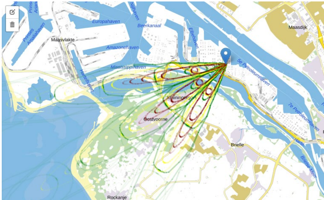
Figure 24 - An ensemble of gas plumes, which shows the operator that there is uncertainty in the direction in which the gas cloud can be moving.
