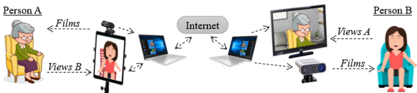
Fig. 1. Overview of the video communication system with AR between the elderly ( Person A ) and the visiting family member ( Person B ). The elderly views the family member projected onto a chair in AR on an iPad Pro, while the visitor views the elderly on a 43" TV screen.
