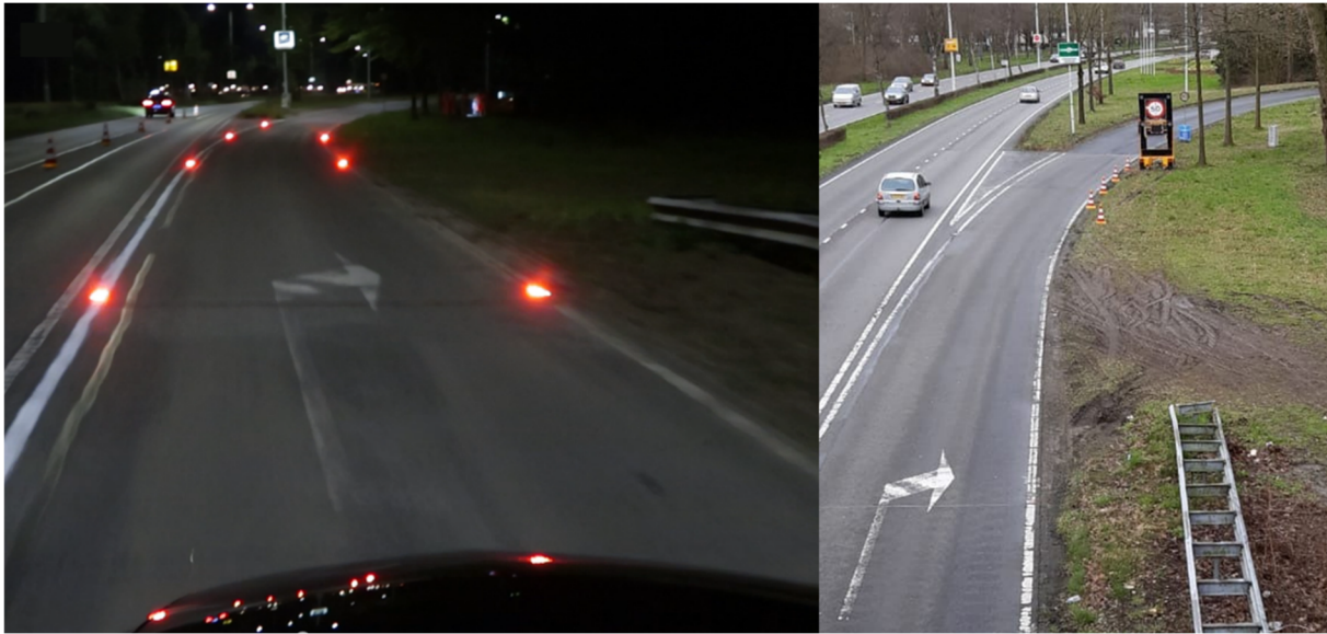
Figure 9-2 On the left: Exemplary view on activated red lights while driving. On the right: Positioning of the speed indicator device.
