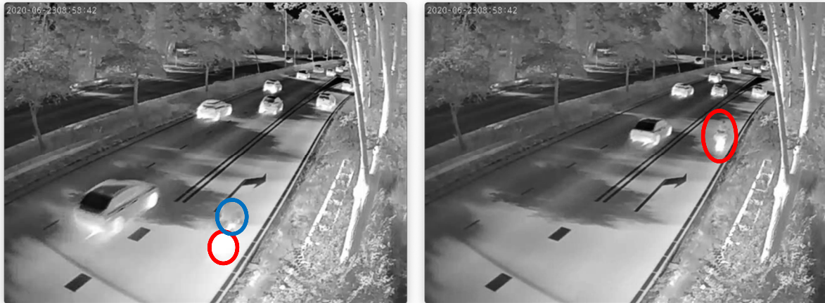
Figure 9-34: Shadows projected on road determines hot and cold spots. On the left image, the engine part (circled in red) and the body part (circled in blue), both hardly visible. On the right image, the whole rider better visible after a few frames.
