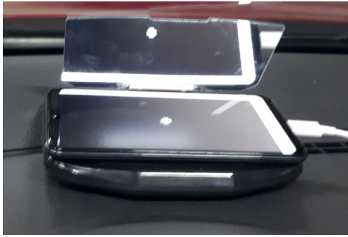
Figure 6-5: Head Up Display consisting of mobile phone and partial transparent mirror
