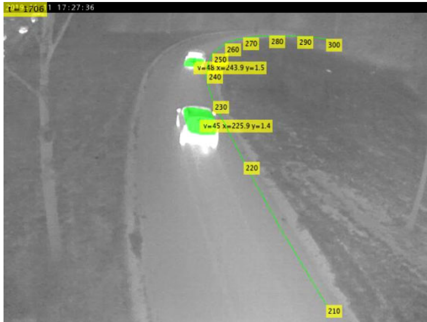
Figure 9-3: Detection of vehicle positions and speed in a road coordinate system, where the x -coordinate is the (longitudinal) position along the road and the y -coordinate is the lateral position, i.e. the orthogonal distance of the vehicle to the right edge of the road.
