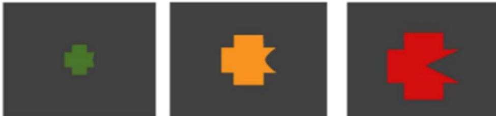
Figure 6.1: Different stages of the HMI escalation. In 30 km/h zones, the small green figure is shown from 50 m before the intersection. The figure evolves into a larger orange cross (30 m before the intersection) to the largest red cross at the intersection. The indent into the cross denotes the direction from which the potential hazard might be expected, in this case from the right.
