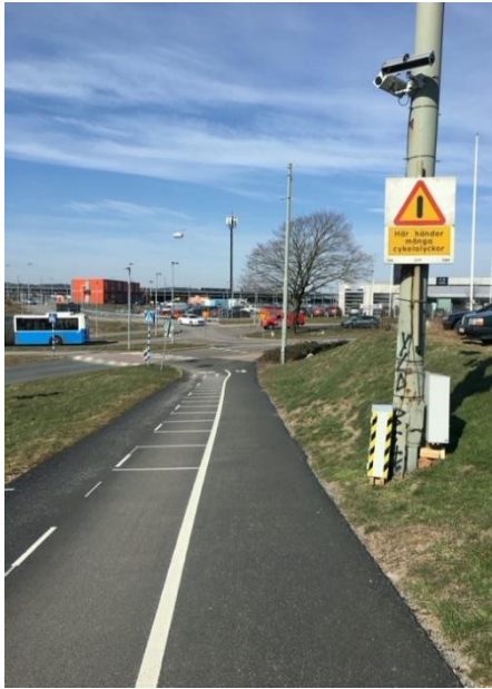
Figure 10.3: Site 2, note the Viscando Otis measuring equipment mounted on the light pole nearest in the picture.
