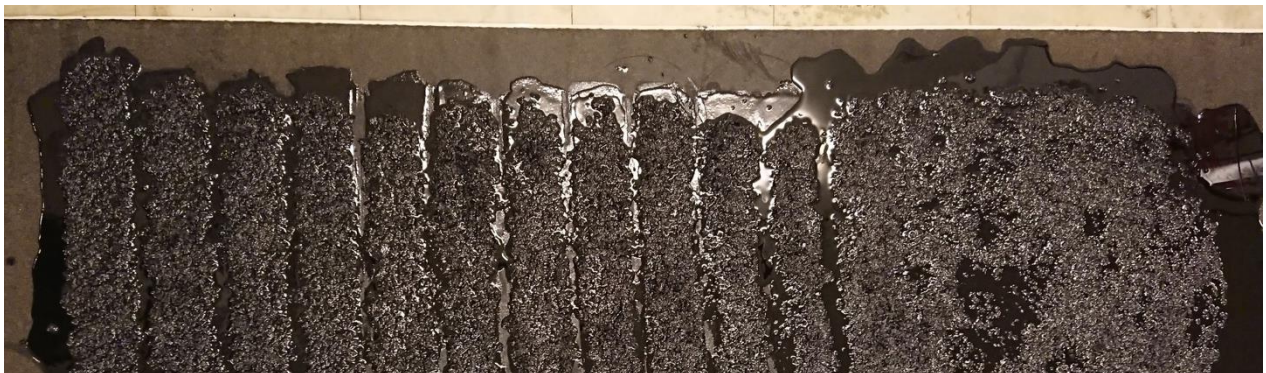
Figure 8-9. An attempt to create 'cut out grooves' in asphalt.
