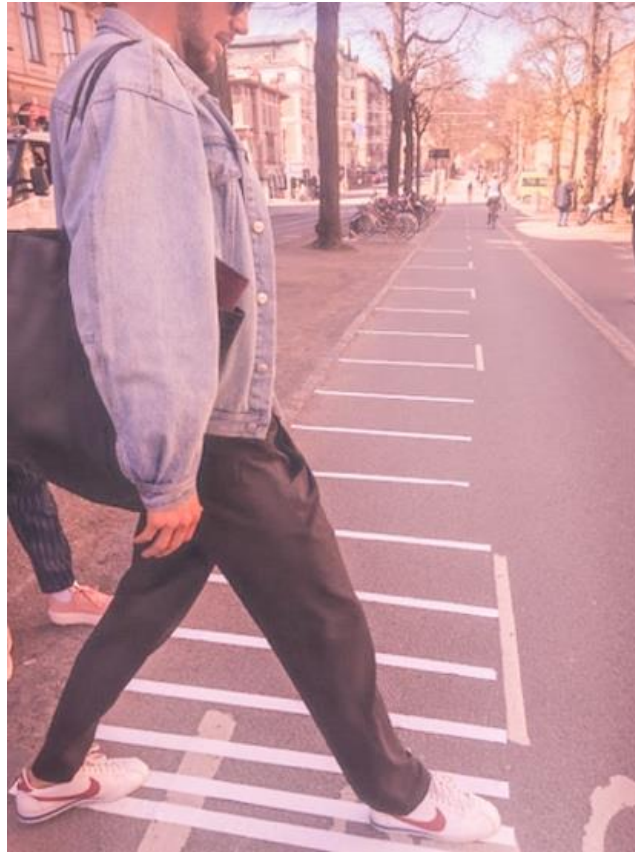
Figure 6-2. Stripes were tested as one way of influencing cyclists' speed.
