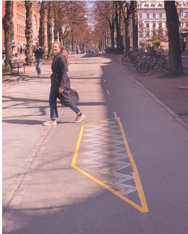
Figure 6-3. Example of narrowing the cycle lane by painting different patterns.
