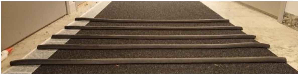
Figure 8-7. Semi-soft rubber strips distributed at a distance of 25 cm.
