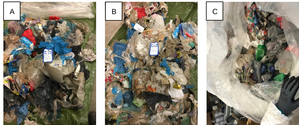
Figure 3.1: The three plastic streams “as received” at TNO: A) DKR310 Small Foils (2D); B) DKR310 Big Foils; C) Mixed Plastics
