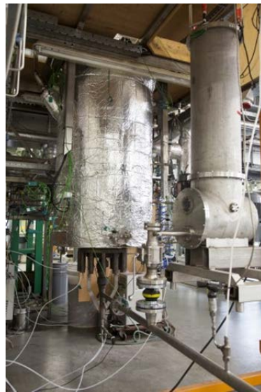
Figure 3.4: Scheme of the lab-scale Milena gasifier (25 kW th )
