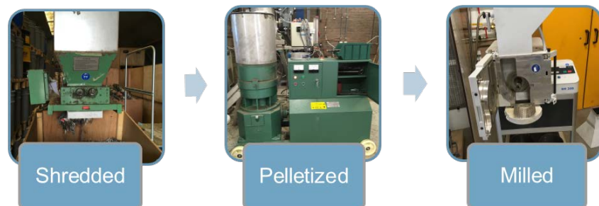
Figure 3.2: Pre-processing of the waste plastic streams prior to the gasification tests
