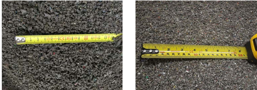
Figure 3.3: Milled plastic streams prior to the gasification tests. Left) DKR310; Right) Mixed Plastics
