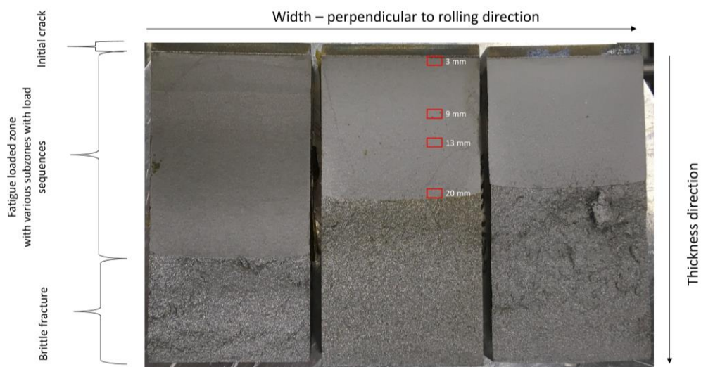
Figure 17a: Fracture surfaces of three base material specimens, BM0835, BM1035 and BM1135
