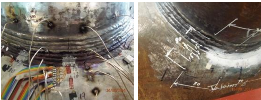
Figure 30: Automated ACPD, reference spacing 15 mm, 1 Amp current
