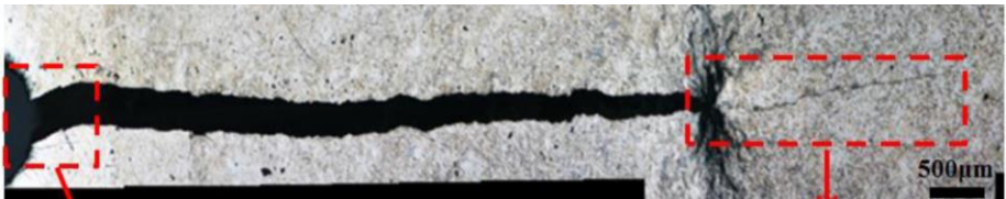
Figure 12: Crack flank before and after an overload, optical microscope image of 304L stainless steel. Image from [59]. Box left-hand side: initiation of the crack from a notch. Box right-hand side: crack flank developed after the overload.
