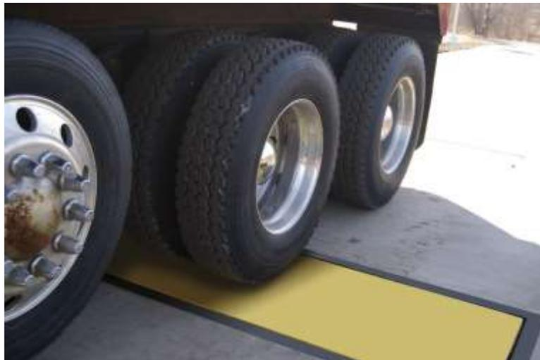
Figure 5.3: Low Speed WIM load plates for measuring the wheel or axle load
