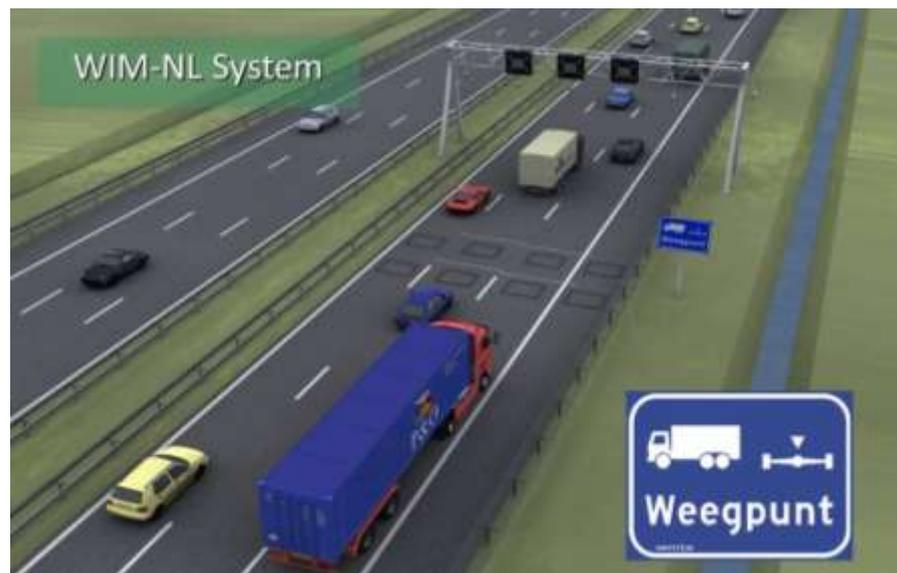
Figure 2.1 WIM-NL system consisting of a combination of in-road sensors and video images
