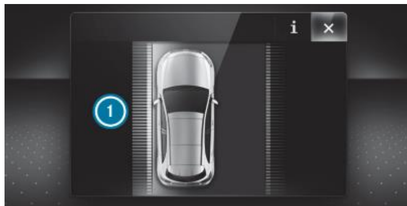
Figure 16 Multifunction display of Mercedes C-Class showing lane-correcting brake application [ID5289].
