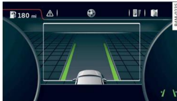
Figure 11 Instrument cluster with Active Lane Assist switched on (left) and Active Lane Assist switched on and active (right) [ID5290].
