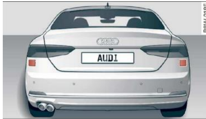
Figure 29 Position of the BSW radar sensors (in red) [ID5290].
