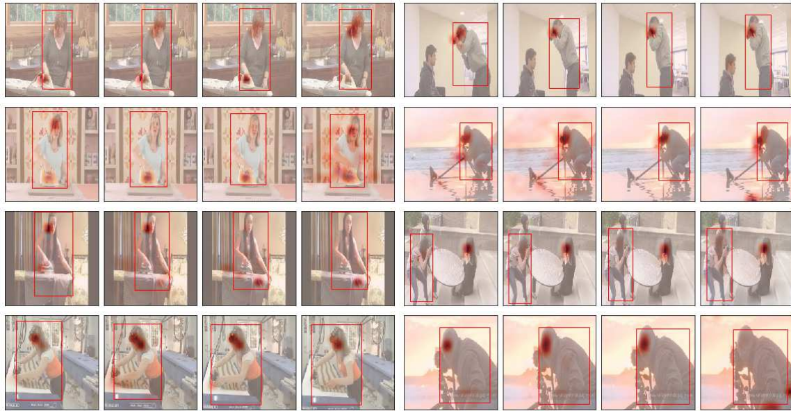
Figure 7: Zero-shot attention maps for classes "Ironing" and "TakingPhotosOrVideos". Although the GCN model has not been trained to recognize these two actions nor their context, it is able to focus on relevant objects. The first two rows illustrate such cases. The last two rows show failure cases, where the attention usually focuses on the actor's head, instead of the object.
