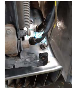
SEMS sensors welded in the vehicle's exhaust
