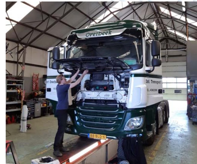
Instrumentation of SEMS measurement system in one of the trucks
