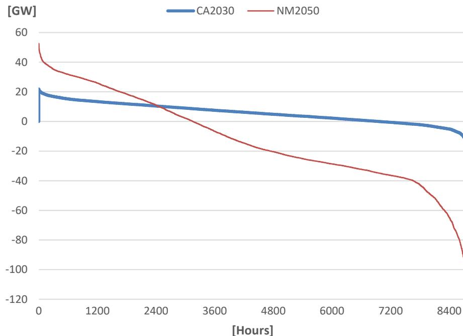
Figure 11: COMPETES: Duration curve of the residual load in CA2030 and NM2050
