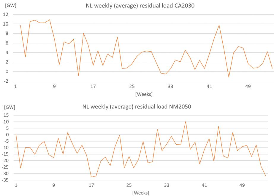
Figure 46: COMPETES: Residual load – Weekly (average) resolution in CA2030 and NM2050
