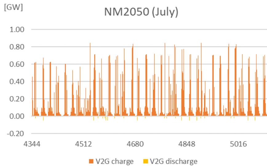
Figure 15: COMPETES: Vehicle-to-grid (V2G) storage transactions in NM2050
