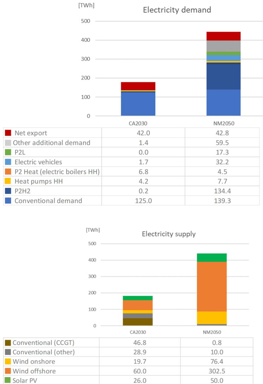
Figure 31: OPERA: Balance of electricity demand and supply in CA2030 and NM2050
