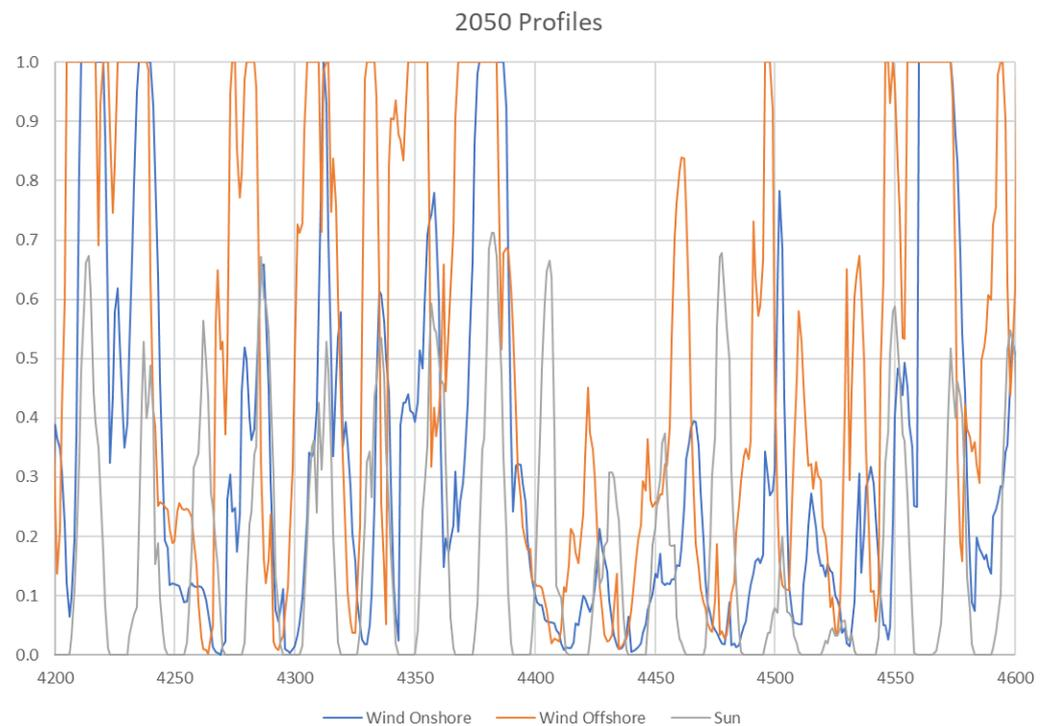
Figure 4: Hourly profiles of the capacity factor for solar PV and offshore wind during the middle of 2050 (hours 4200 – 4600)
