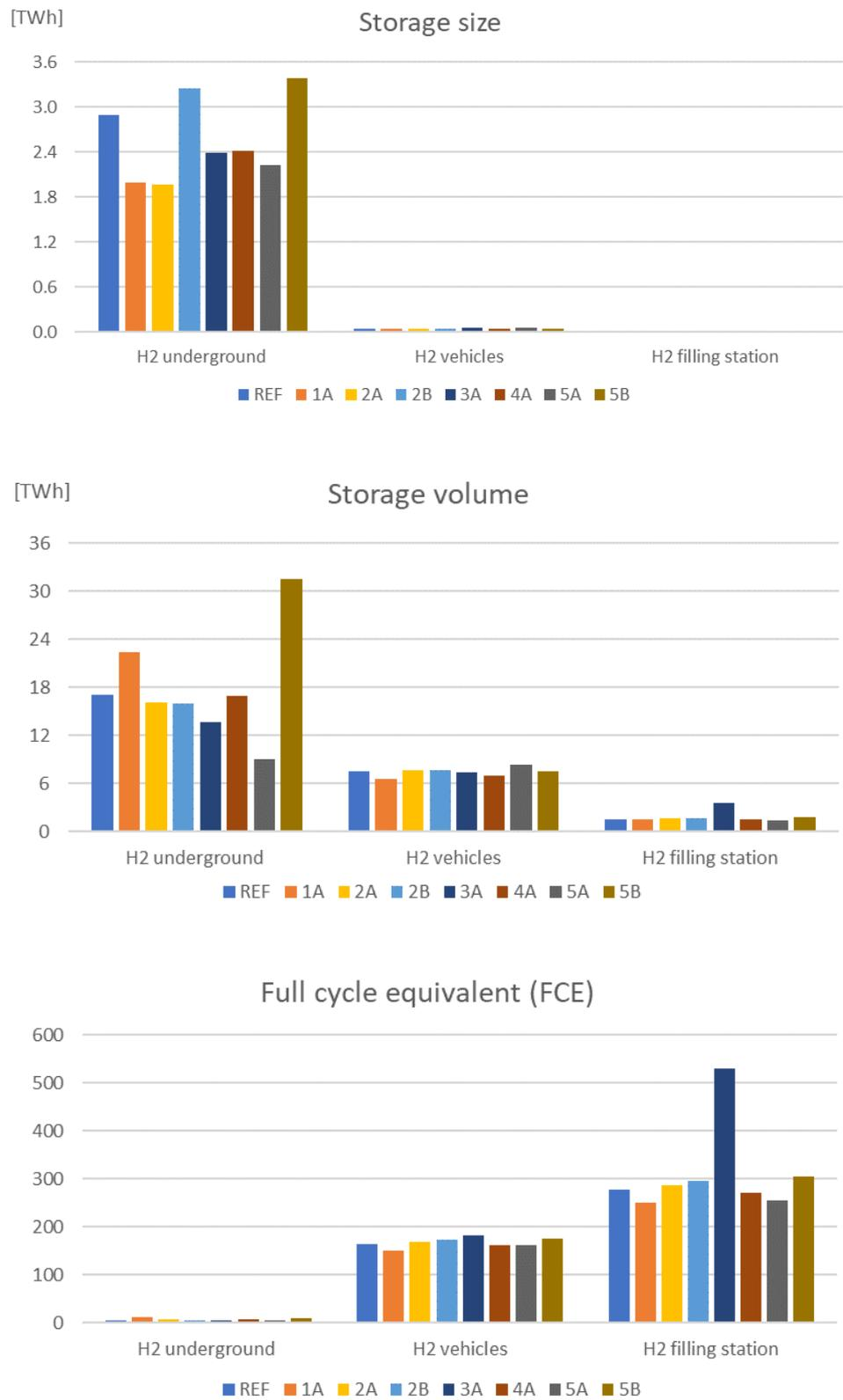
Figure 43: OPERA: Hydrogen storage results – Comparison of NM2050 reference scenario and sensitivity cases
