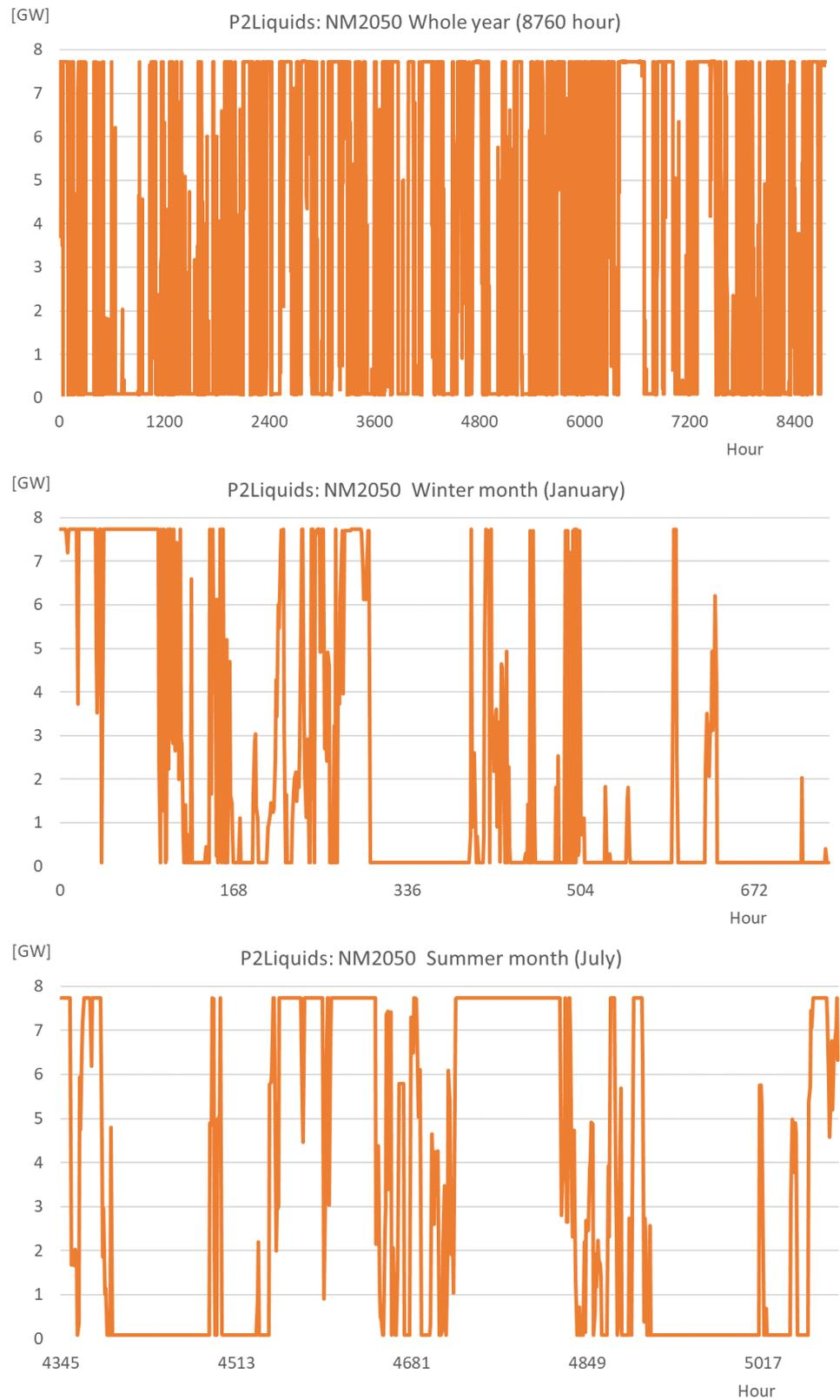
Figure 52: OPERA: Hourly profiles of H<sub>2</sub> demand by Power2Liquids in NM2050
