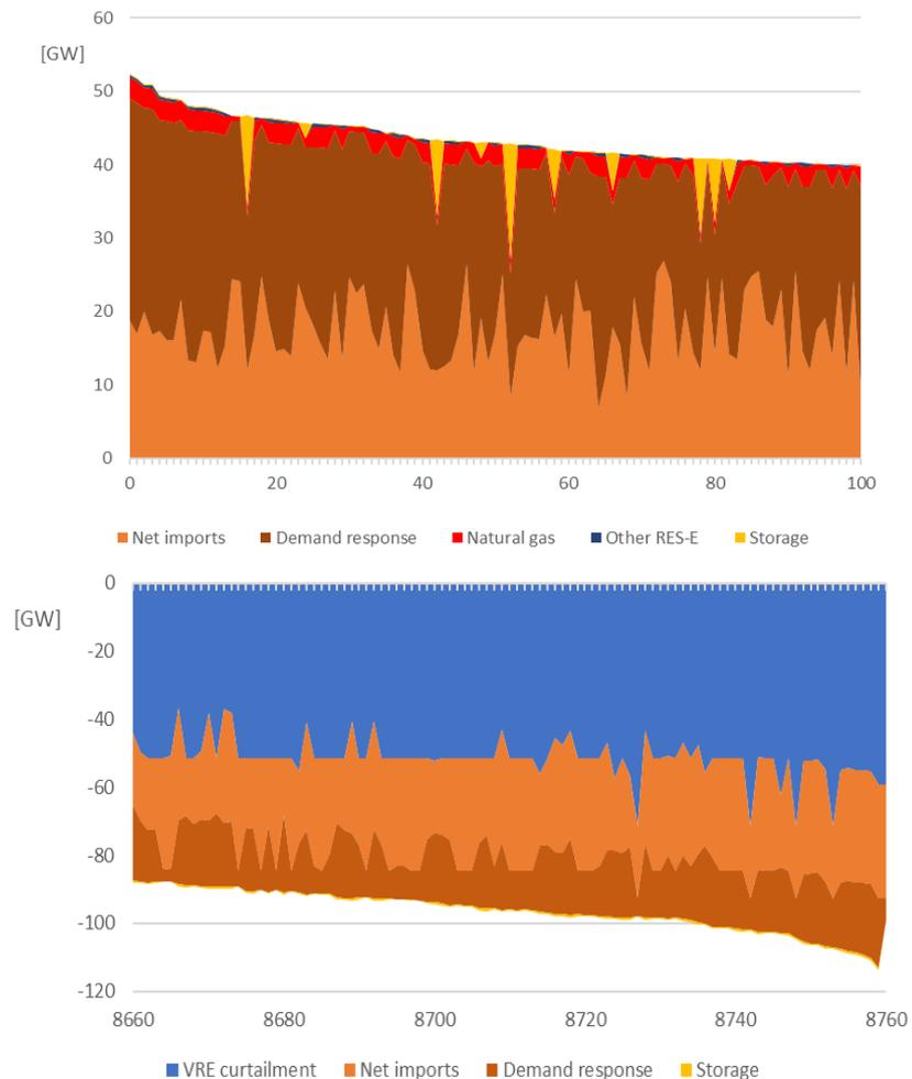
Figure 12: COMPETES: Flexibility options during the first 100 ('peak') and last 100 ('off-peak') hours of the residual load duration curve in NM2050
