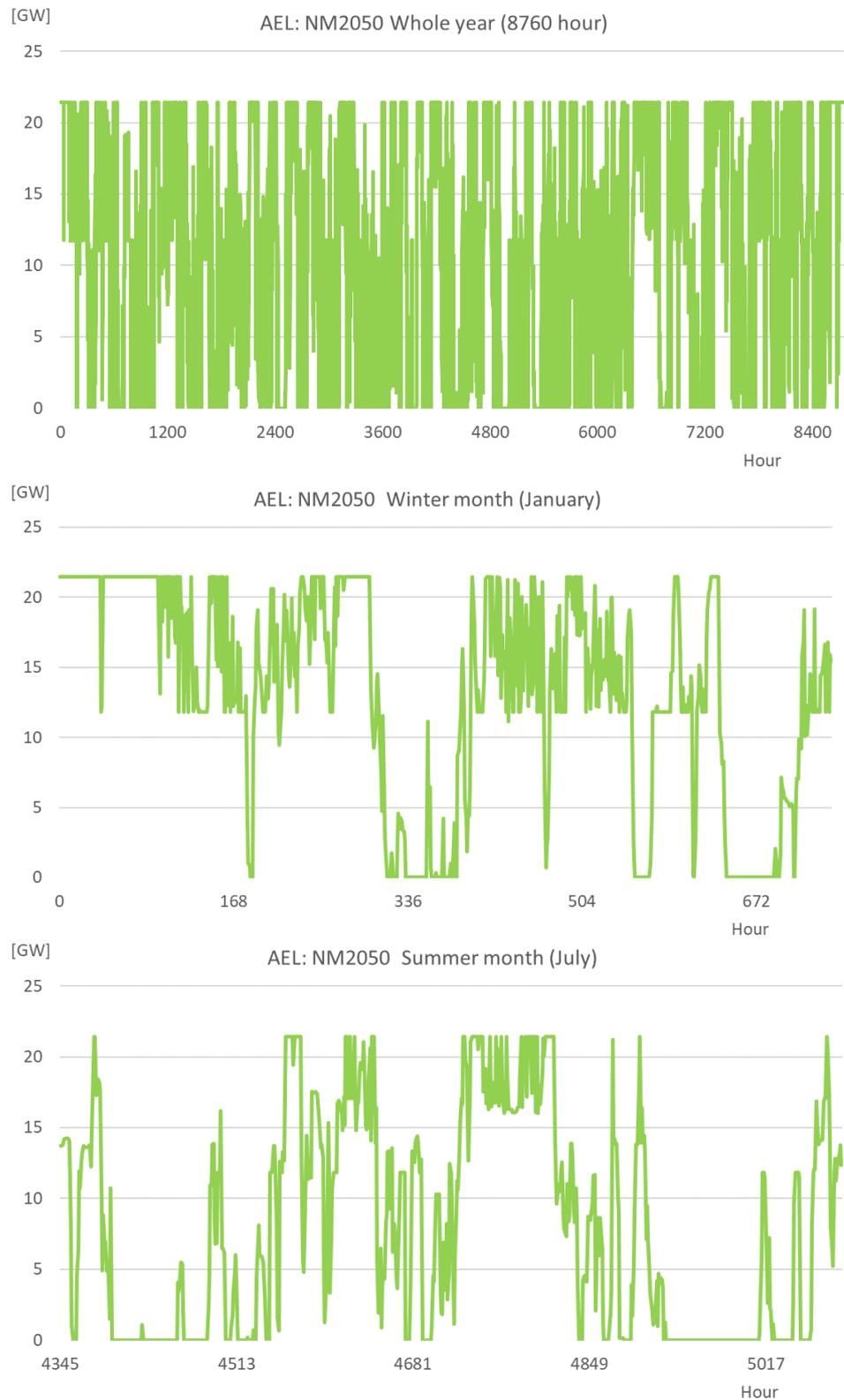
Figure 53: OPERA: Hourly profiles of H<sub>2</sub> supply from alkaline electrolysis (AEL) in NM2050
