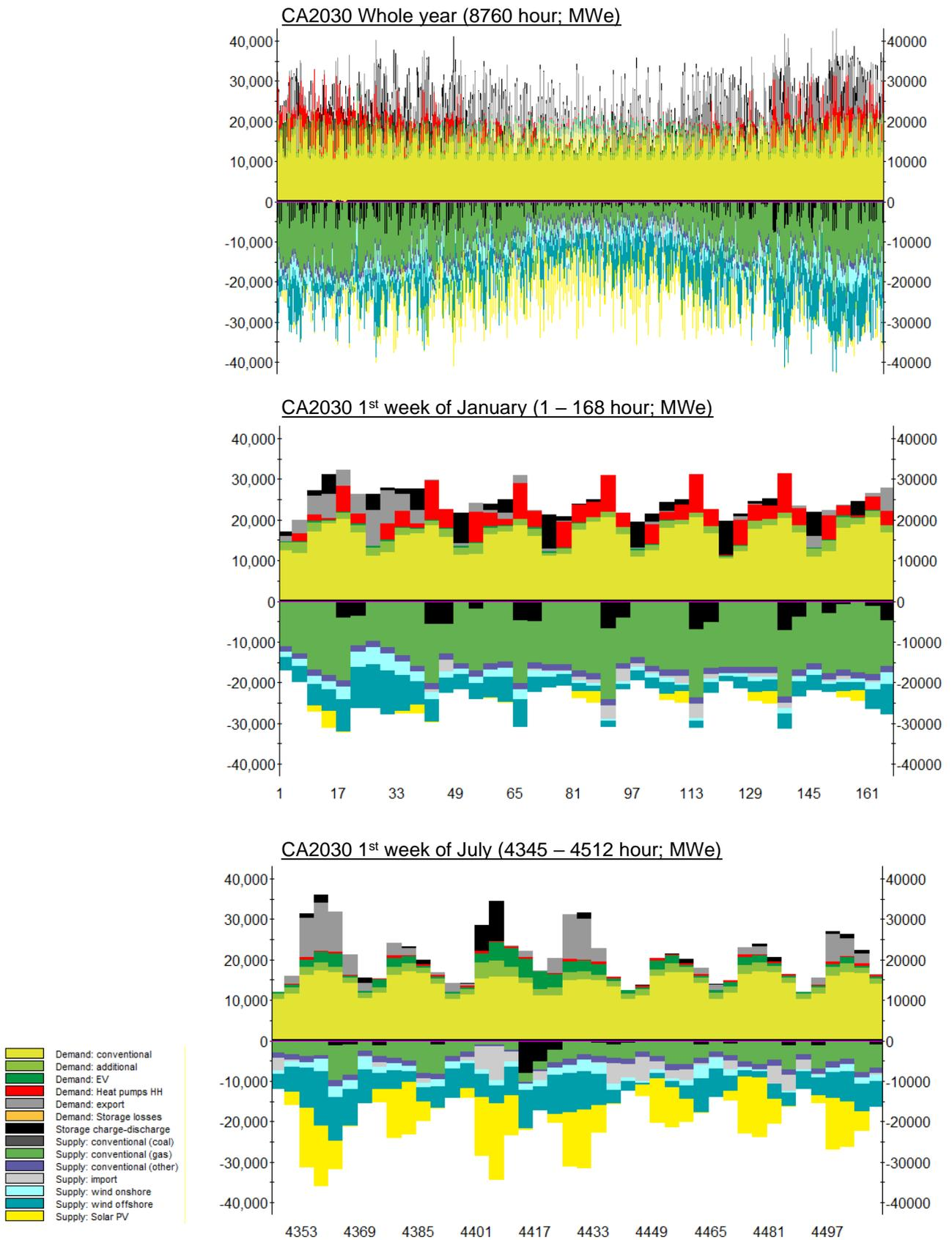
Figure 33: OPERA: Hourly electricity profiles in CA2030
