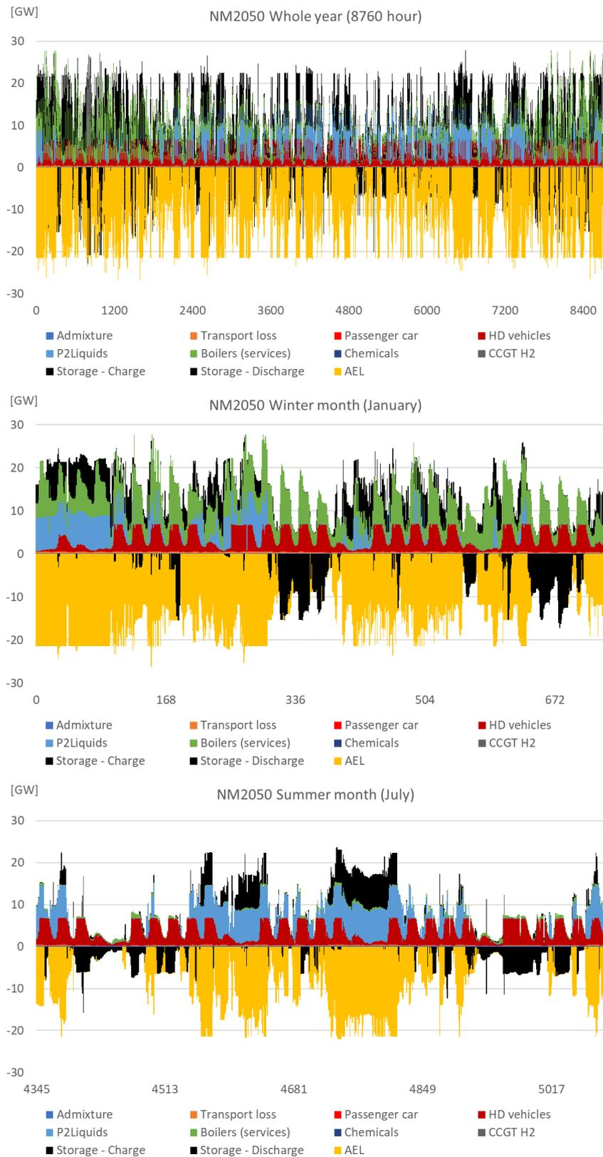
Figure 36: OPERA: Cumulative hourly profiles (stacked columns) of different categories of H<sub>2</sub> demand, supply and storage in NM2050
