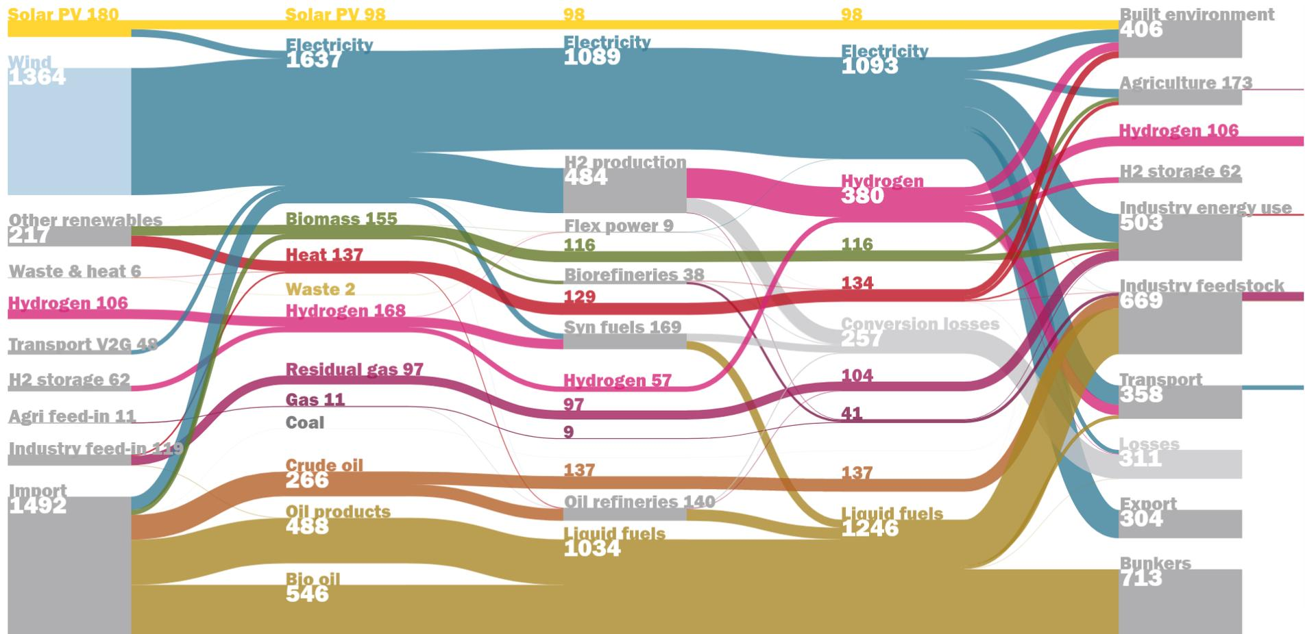
Figure 56: OPERA: Sankey diagram of the energy system in the Netherlands in NM2050
