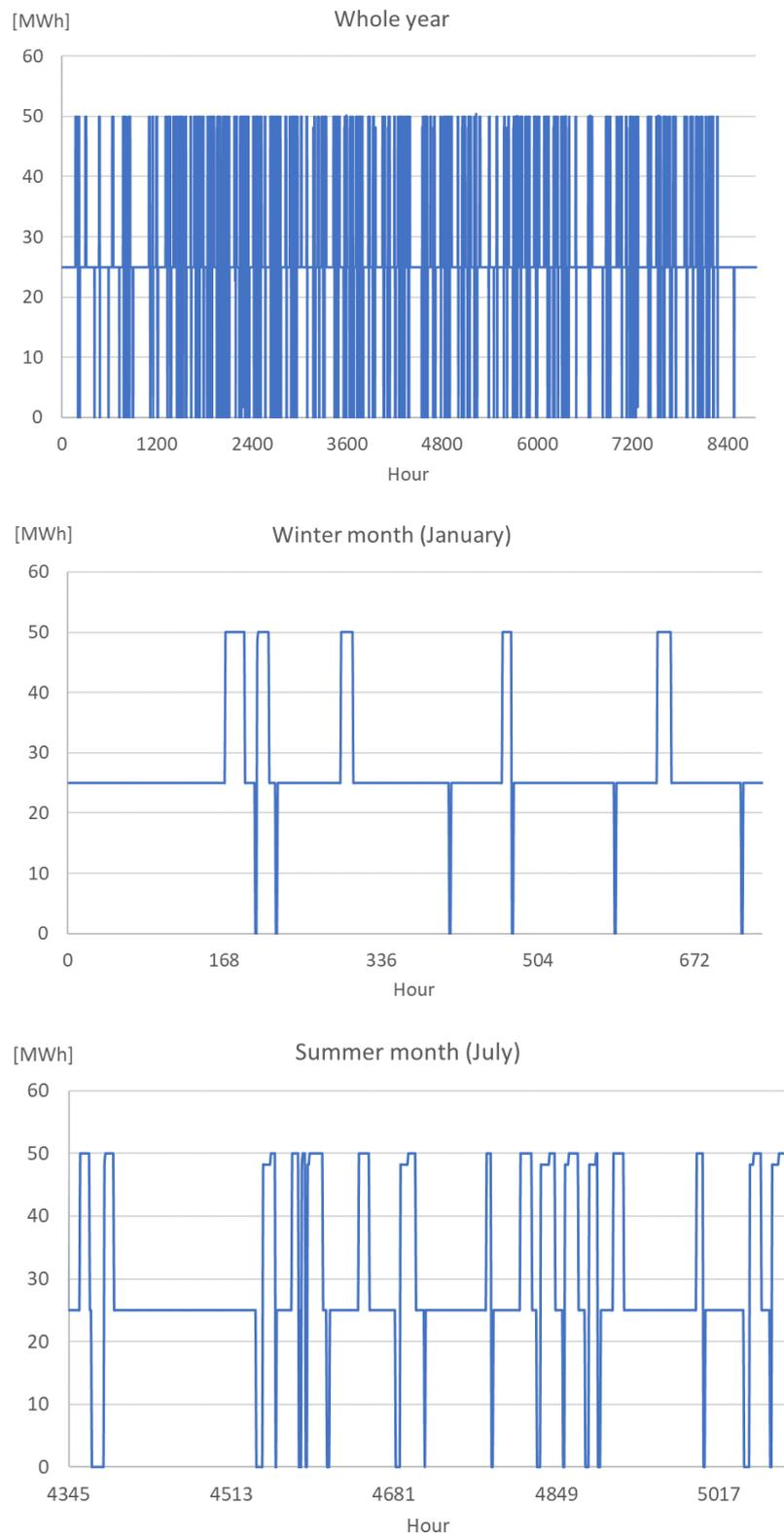
Figure 17: COMPETES: State of charge of electricity storage by Li-ion batteries in NM2050
