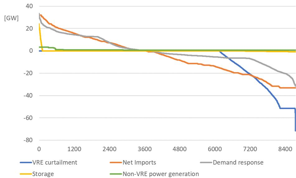
Figure 14: COMPETES: Load duration curves of flexibility options in NM2050
