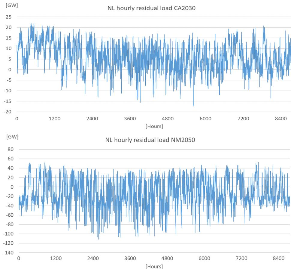
Figure 10: COMPETES: Residual load – Hourly resolution in CA2030 and NM2050
