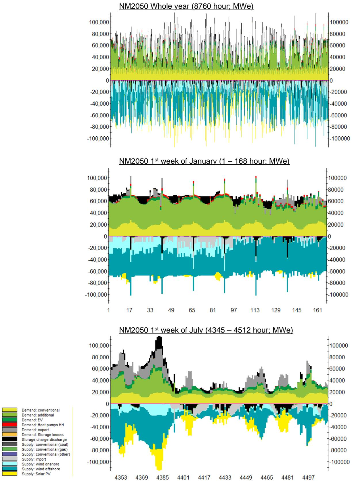
Figure 34: OPERA: Hourly electricity profiles in NM2050
