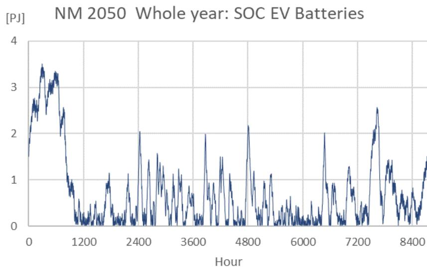
Figure 35: OPERA: State of charge of the EV batteries in NM2050
