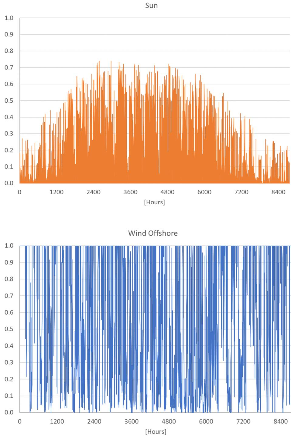
Figure 44: COMPETES and OPERA: Hourly profiles of the capacity factor for solar PV and offshore wind during the whole year 2050 (8760 hours)
