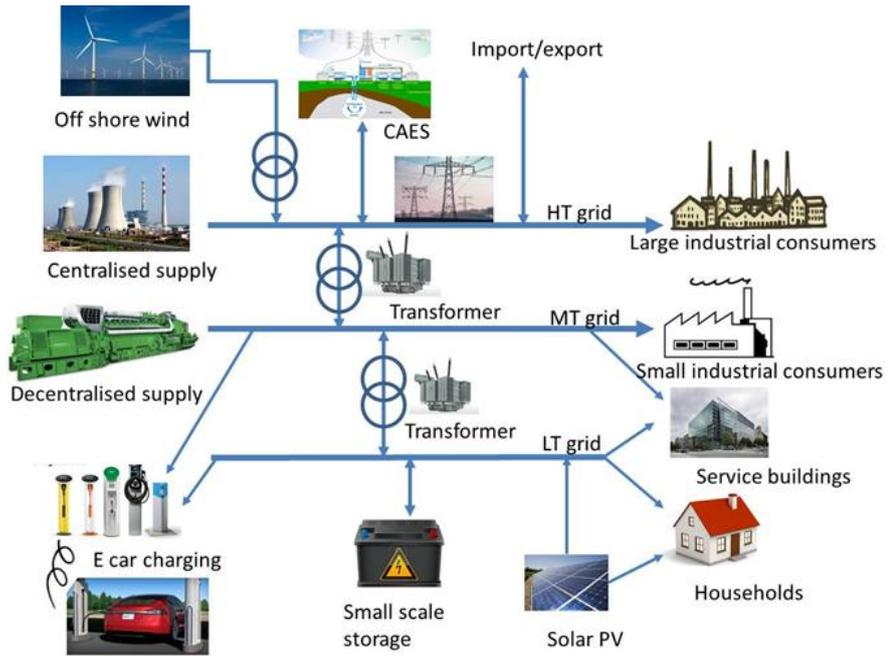
Figure 2: Schematic illustration of the electricity system represented in OPERA, including electricity infrastructure and storage
