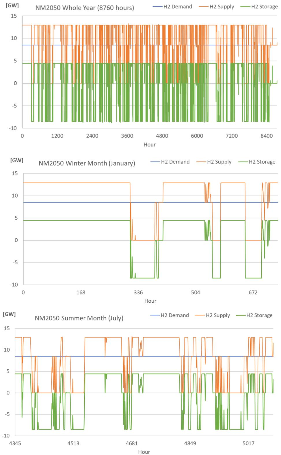
Figure 19: COMPETES: Hourly profiles of H<sub>2</sub> demand, supply and storage in NM2050
