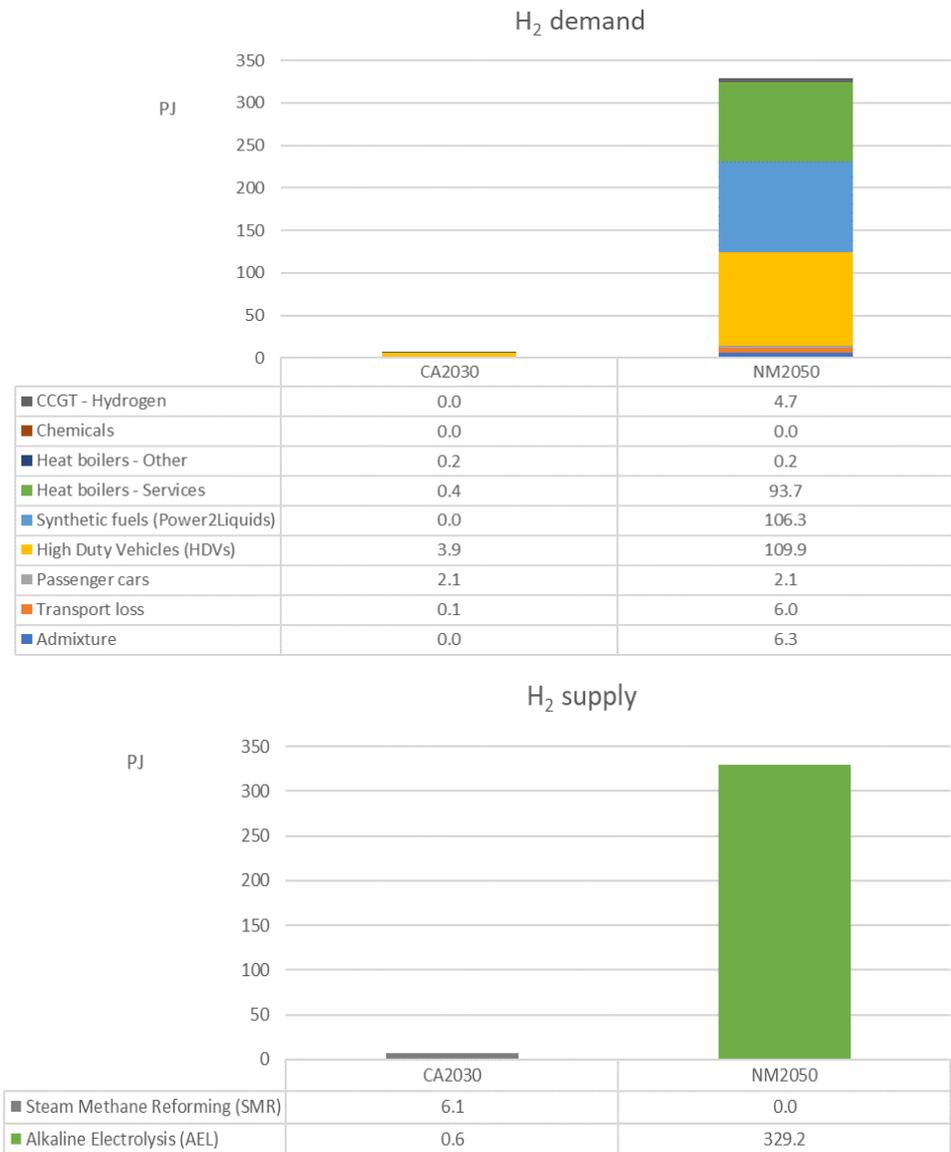
Figure 32: OPERA: Balance of hydrogen demand and supply in CA2030 and NM2050
