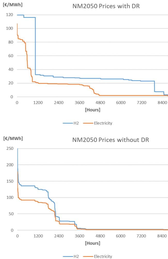
Figure 22: COMPETES: Duration curve of hourly electricity and hydrogen prices in NM2050 (with and without demand response)
