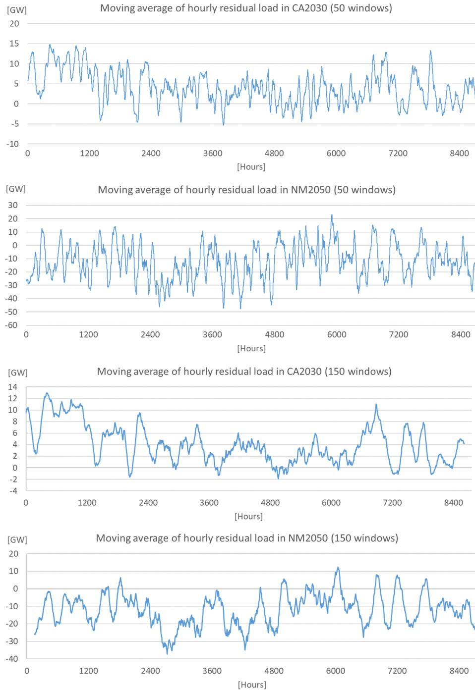
Figure 47: COMPETES: Moving average of hourly residual load over 50 and 150 windows in CA2030 and NM2050
