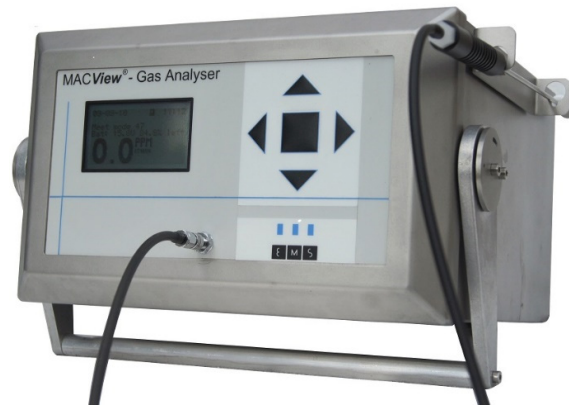
Figure 13: Ethylene gas measurement sensor with O 2 and CO 2 sensors, MACView® post-harvest gas analyser from Environmental Monitoring Systems (EMS). The device is based on an electrochemical ethylene gas sensor with an accuracy down to 0.1 ppb [20]. Picture: courtesy of EMS.
