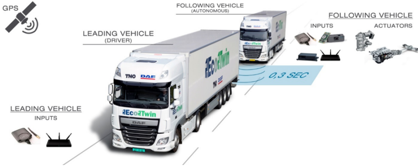
Figure 7.3: EcoTwin truck platooning concept
