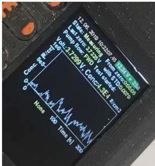
Figure 3-12: DPF inspection tool in action
