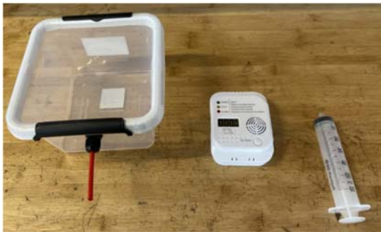
Figure 3-1: CO meter test equipment
