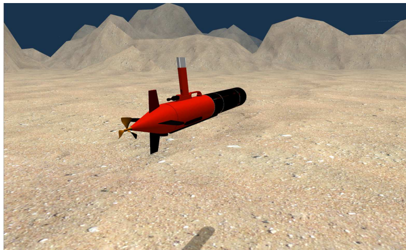
Figure 4-7: Screenshot of the UUV Simulator visualisation with the virtual LAUV
