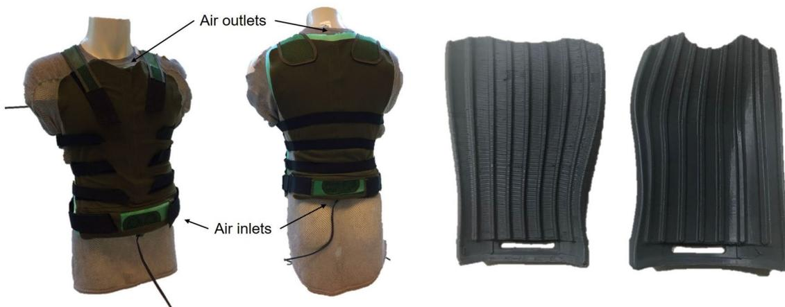
**Fig. 1** Ventilating vest. Ventilators at the air inlets allow for the flow of air through channels in the vest. On the left, the vest is shown from the outside, on the right the vest is shown from the inside. The venti-
