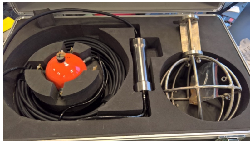
Figure 2.3 Overview of the vector sensor (orange sphere), signal conditioner with pre-amplifiers (steel cylinder) and suspension cage (right).
