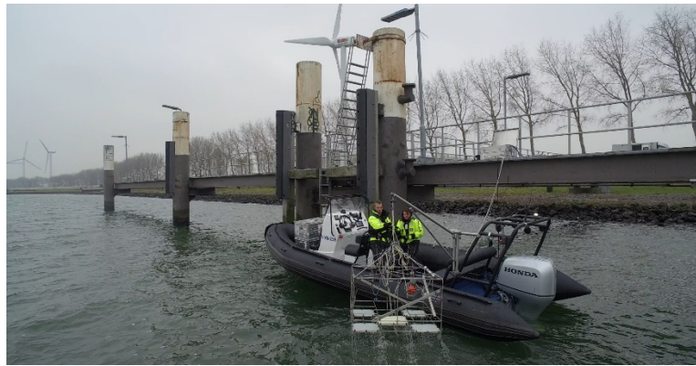
Figure 5.2 Recovery of the vector sensor at the cage at the Haringvliet inland waterway.
