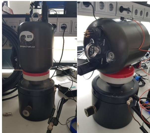
Figure 4.13 M20 Vector sensor installed on an electro dynamic shaker in various directions.
