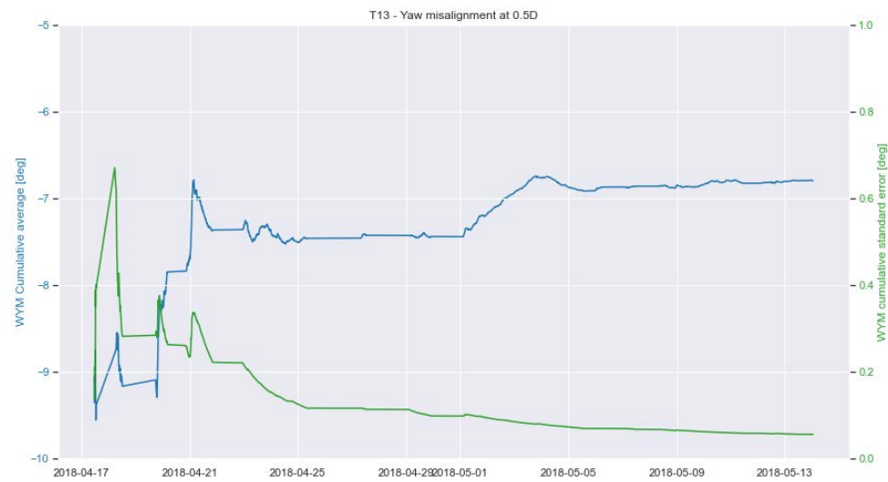
Figure 22 Cumulative average yaw misalignment for turbine 13 (campaign a).
