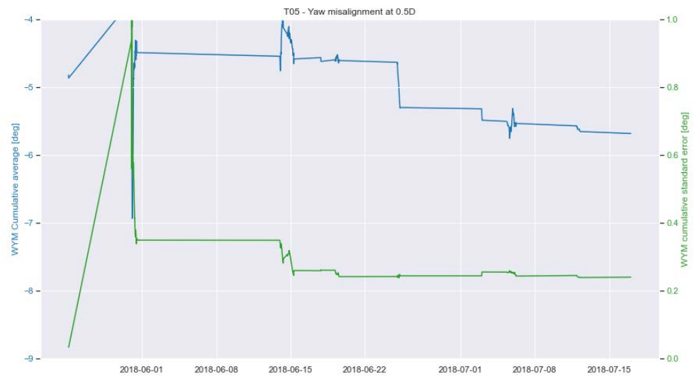
Figure 24 Cumulative average yaw misalignment for turbine 5.
