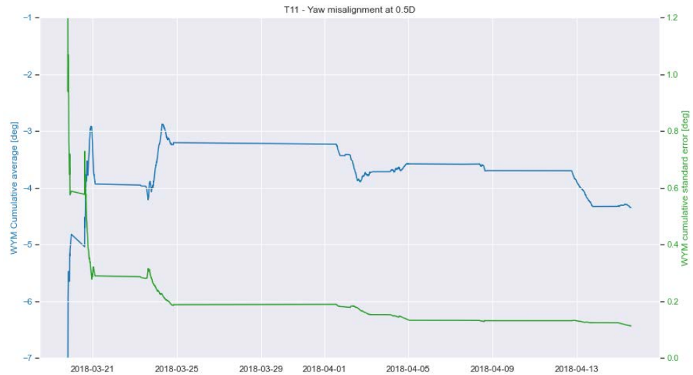
Figure 20 Cumulative average yaw misalignment for turbine 11.
