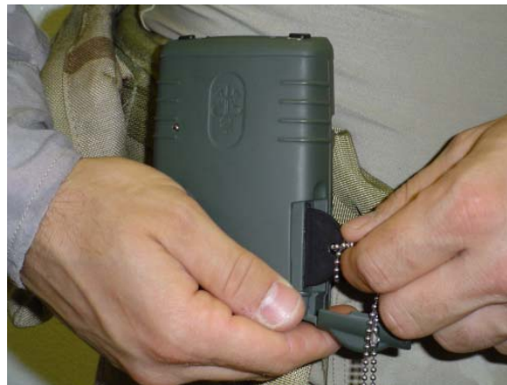
Figure 2-4: WPSM-IC Computational Center (Hub), Showing the Insertion of the Personal Information Carrier (PIC – A Memory Card Containing Medical Records and Personalization Information for the Algorithms). Once the PIC is inserted, the hub will be keyed to an individual and the personal information used to personalize the models and classifiers.
