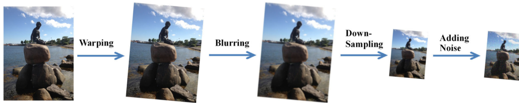
FIGURE 1.2: The imaging model employed in most SR algorithms. Nasrollahi and Moeslund, 2014.
