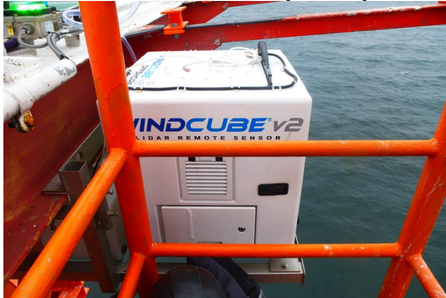
Figure 8 Installed LiDAR (side view with safety net removed)
