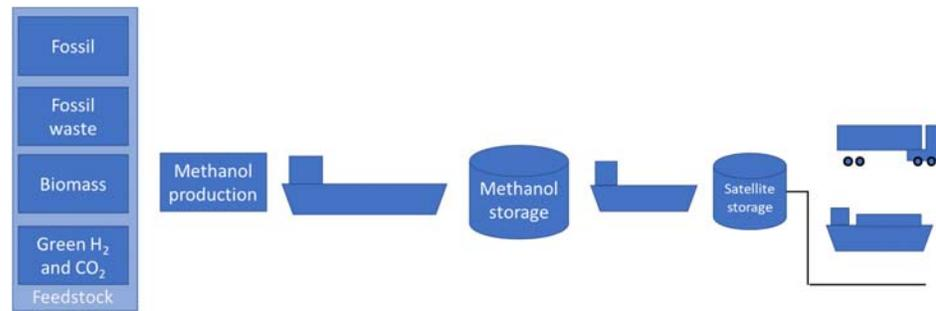
Figure 1: Supply chain of methanol as a maritime fuel.
