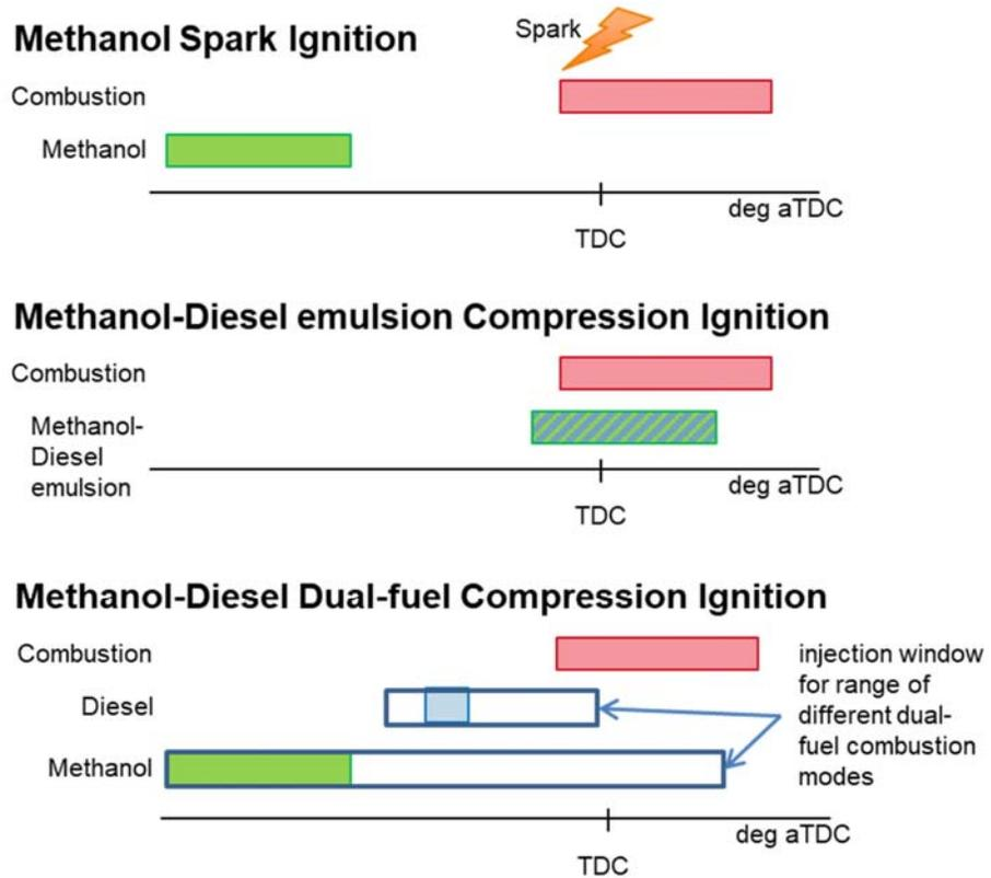
Figure 5: Three combustion technologies for use of methanol in engines. The x-axis is the time represented by the engine crank angle relative to the piston Top Dead Center (TDC). The coloured blocks mark the fuel injections and the combustion process in time.
