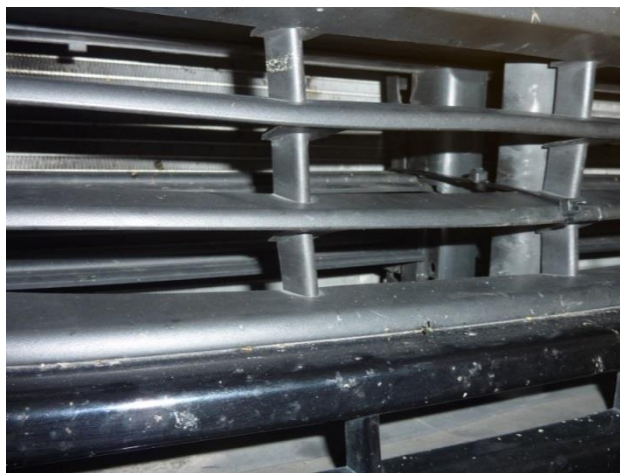
Figure 46: Active grill vanes in open position
