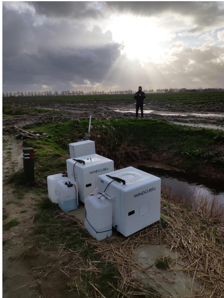
Figure 7: The Leosphere WLS7-258 LiDAR
