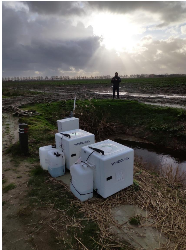
Figure 7: The Leosphere WLS7-258 LiDAR
