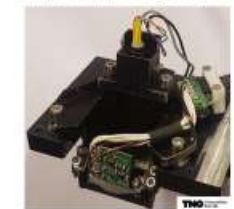
Figure 2: LDR-AFM head mountable on the 6-DOF Hexapod stage.
